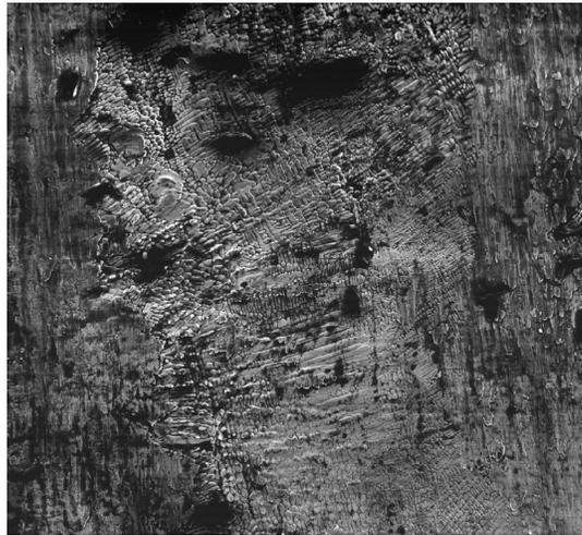
Figure 11. Hot cracking behaviour, industrial tube welding line, clad Alloy 800, filler Alloy 625
