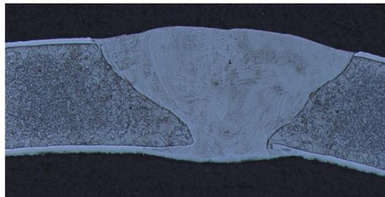
Figure 5. Shape of laser weld, industrial tube welding line
