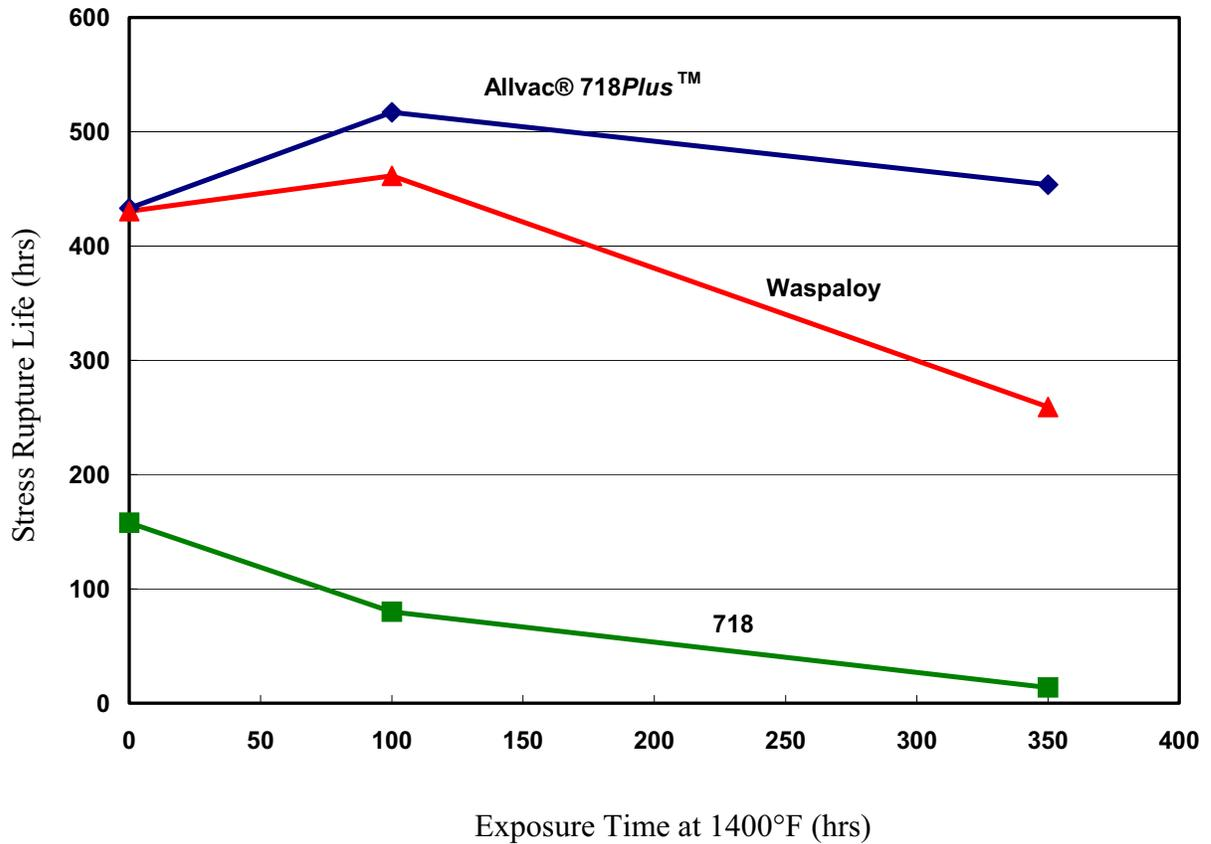
Figure 3. Effect of Thermal Exposure on Rupture Life at 1300°F/80 ksi.
