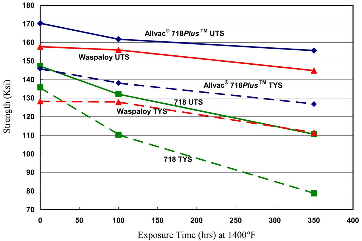
Figure 2. Effect of Thermal Exposure on Ultimate Tensile and Yield Strength at 1300°F
