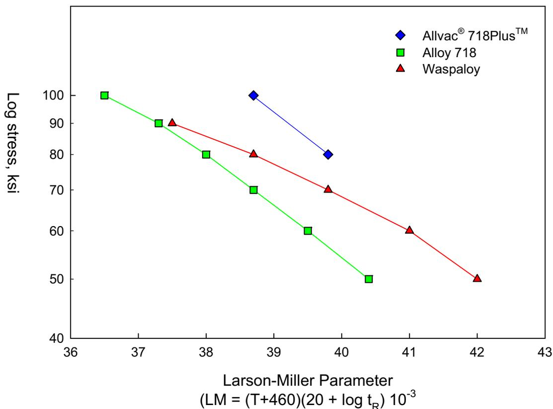
Figure 1. Larson-Miller Stress Rupture Life Comparison
