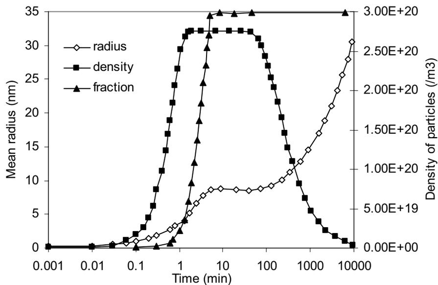
Figure 3. Calculation of time evolution of mean radius, precipitate fraction and density of particles for a steel of composition  $105 \times 10^{-3} \text{wt}\% \text{Nb}$ ,  $9 \times 10^{-3} \text{wt}\% \text{C}$  aged at  $700^\circ \text{C}$ .
