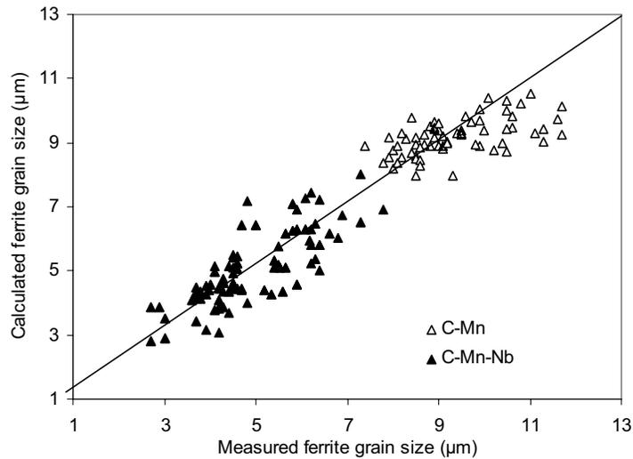
Figure 2. a) The effect of residual strain in the austenite through the effective austenite grain size on final ferrite grain size is schematically described. b) The simplified approach for grain size prediction gives good agreement with experimental measurements.
