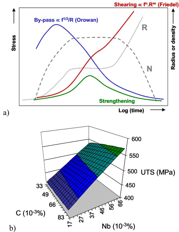
Figure 4. a) Schematic view of the precipitation strengthening curve as a function of isothermal soaking time due to the mechanism changes from looping to shearing when the mean precipitate radius increases. b) Calculations according to the multi-precip model show a linear dependency of the strengthening peak height with Nb content, while C content has nearly no effect.
