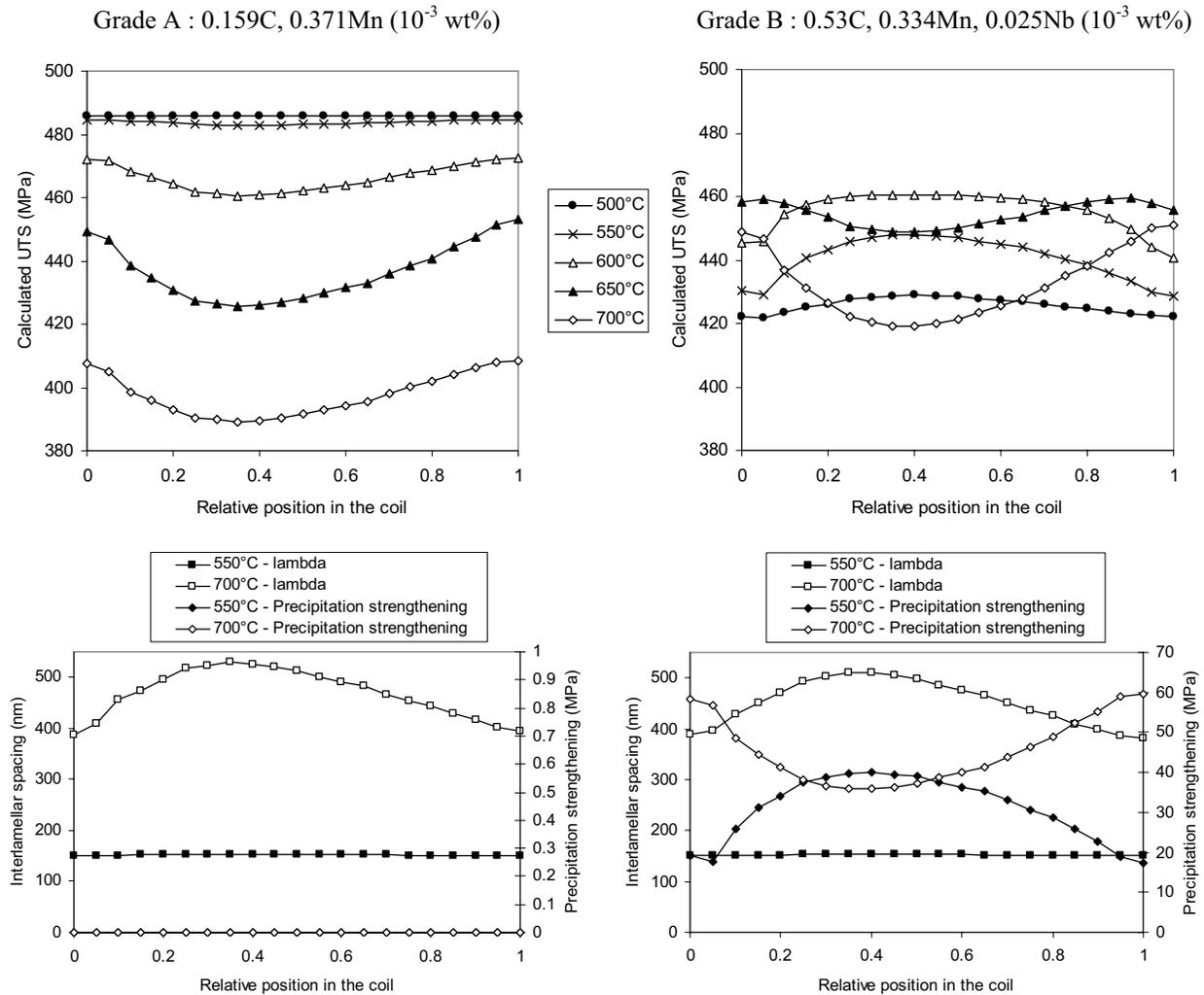
Figure 8: a) The profile of ultimate tensile strengths over the entire strip length strongly depends on the chemistry and on the coiling temperature. b) Modelling enables to visualise the various sources of strengthening and heterogeneity through the coil: precipitation strengthening for microalloyed steels, pearlite softening for “high pearlite” containing grades, described as an increase of interlamellar spacing  $\lambda$ .
