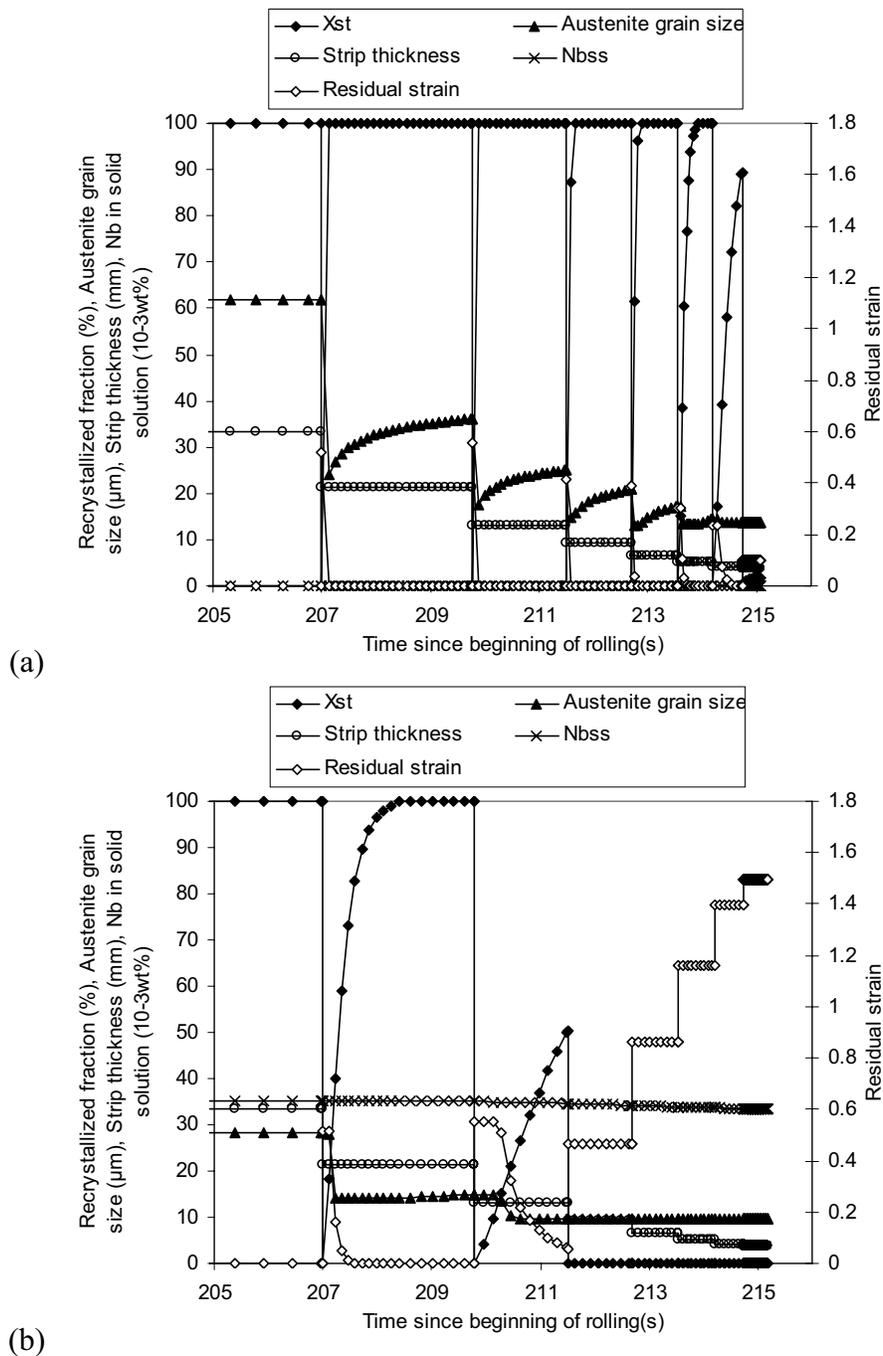
Figure 1. Evolution of austenite microstructure in the finishing mill according to FAST model for a) Grade A: C75, Mn300 (10<sup>-3</sup> wt%), b) Grade B: similar to A + 35 · 10<sup>-3</sup> wt%.
