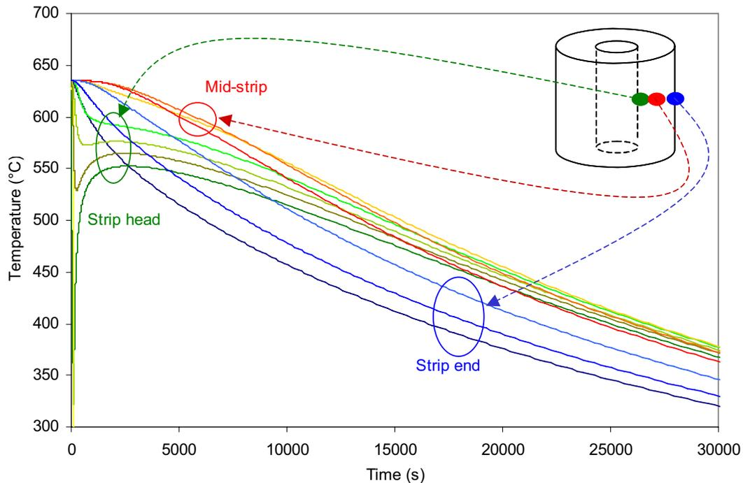
Figure 6. Thermal evolutions at ten different positions in the coil according to a 2-dimension thermal model of the coil, characterised by an imperfect thermal contact between the wraps [15].
