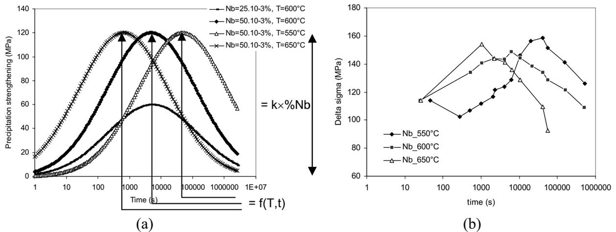
Figure 5. Precipitation strengthening curve according to Militzer approach [13]: the position of the peak, which strongly depends on the thermal path is fitted on experimental isothermal holding (due to Militzer also [13]); the height of the peak is fitted according to results from Multi-precip model shown in Figure 4b.
