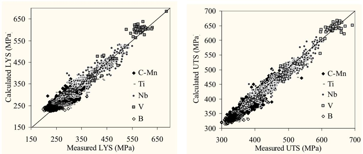
Figure 7: Prediction of the lower yield strength and of the ultimate tensile strength by TACSI for C-Mn, HSLA and drawing hot rolled strips. The accuracy around 13MPa for UTS is very satisfactory.
