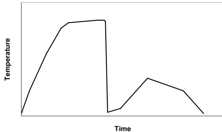
Figure 3. Typical time and temperature cycle for a dual phase grade.
