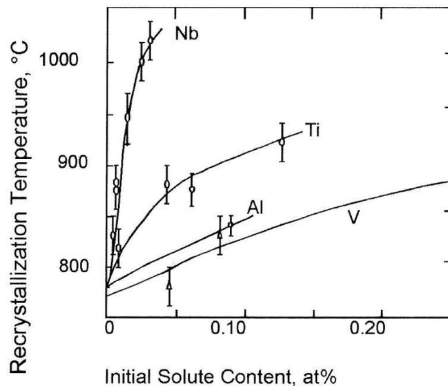
Figure 1. The increase in recrystallization temperature with different microalloying elements in a 0.07C, 1.40Mn, 0.25Si steel [1].
