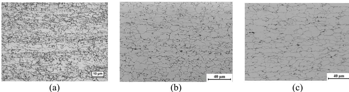
Figure 4. Typical microstructure of Nb-alloyed steel grades: (a) Domex 700 MC, (b) Docol 420 YP, (c) Dogal 350 YP.
