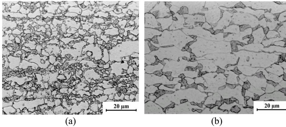
Figure 5. Microstructure of dual phase steels:
