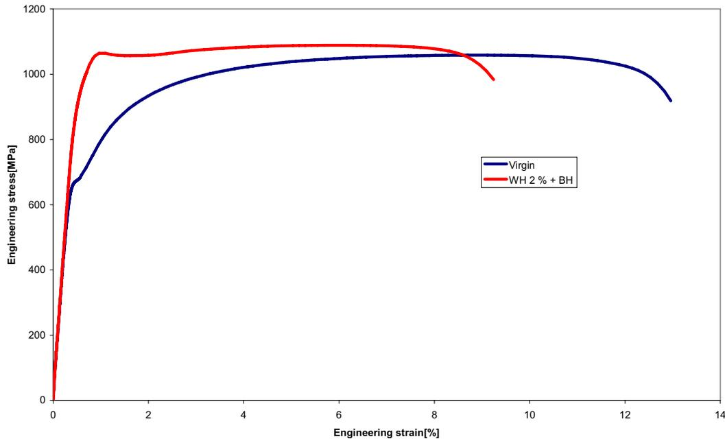
Figure 11. Engineering stress versus engineering strain for Docol 1000DP.
