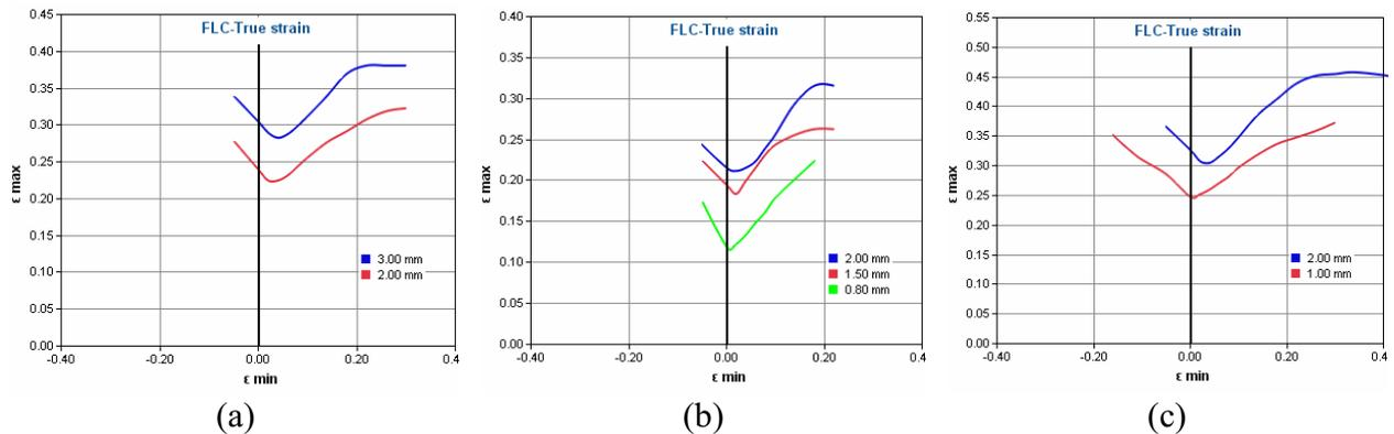
Figure 7. Typical forming limit curves for Nb-alloyed steel grades [4]:
