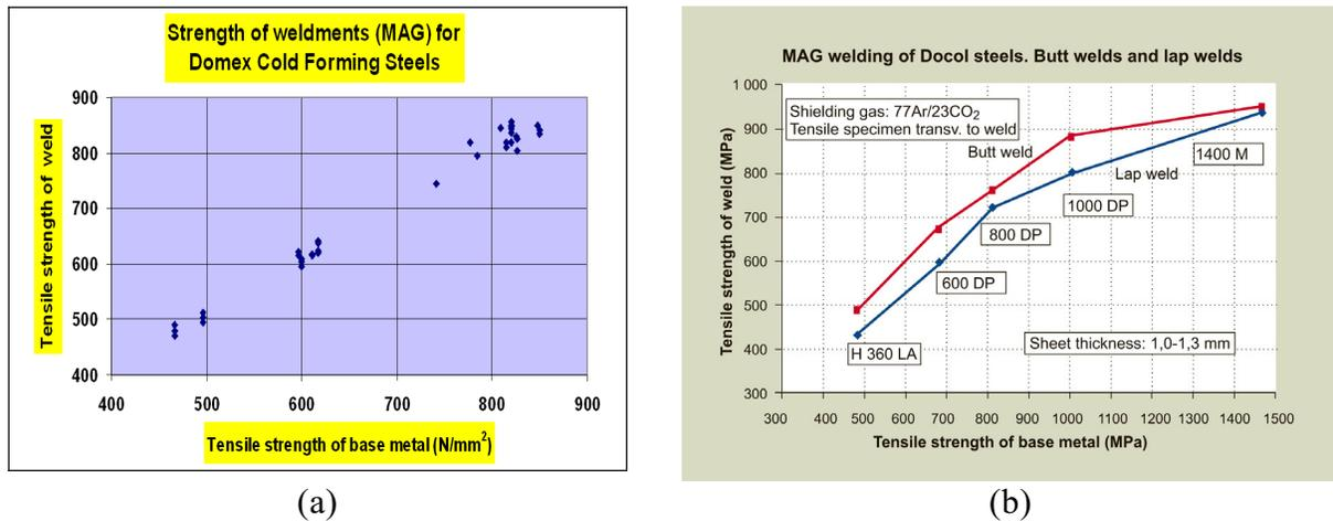
Figure 9. Tensile strength of MAG weld as a function of tensile strength of base metal for (a) Domex microalloyed cold forming steels. Butt welds, matching electrodes have been used. (b) Docol microalloyed, dual phase and martensitic steels. Butt and lap welds.
