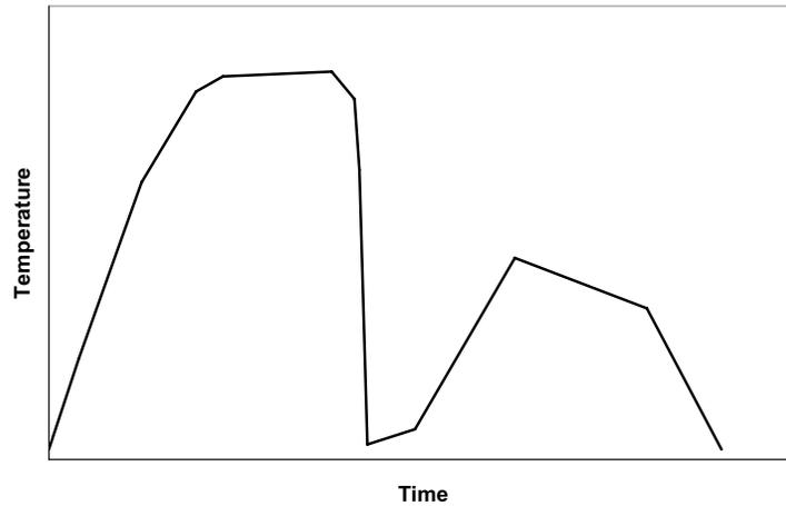
Figure 2. Typical time and temperature cycle for a microalloyed grade.
