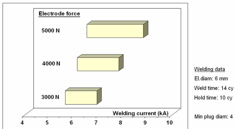
Figure 8. Typical spot welding parameters for spot welding Docol 1000 DP 1.20 mm to itself. Failure mode is full plug failure.
