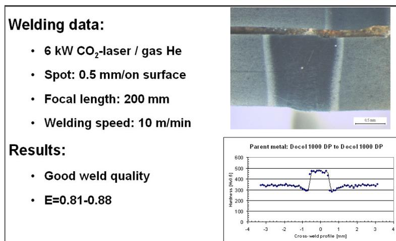
Figure 10. Formability results and hardness profile of typical laser weld in Docol 1000 DP 1.20 mm. E=Erichsen value expressed as formability of the weld divided with formability of the base metal.
