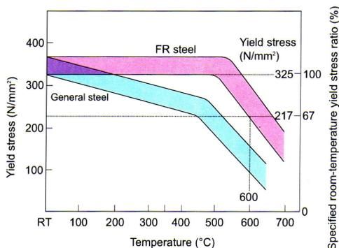
Figure 1. Schematic comparison of improved elevated temperature strength of FR steel. (Adapted from [1], with permission).
