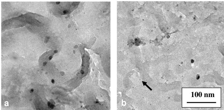
Figure 6. TEM bright field images from carbon extraction replicas showing fine precipitates in the Nb (a) and Mo+Nb (b) alloys after constant load testing at 300°C/hr [2].
