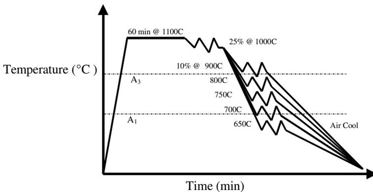
Figure 8. Schematic illustration of thermomechanical processing variations used to examine the influence of warm working in Nb-containing steel [24].
