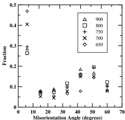
Figure 9. Distribution of misorientation angles for Nb steel laboratory rolled using finishing temperatures between 900°C and 650°C.
