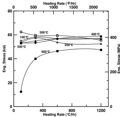
Figure 4. Influence of heating rate (100°C/Hr – 1200°C/Hr) to test temperature on the yield strength of the Mo+Nb alloy. Testing was conducted at an engineering strain rate of about  $3.9 \times 10^{-3} \text{ s}^{-1}$  following a 15 minute holding time at the test temperature [19].
