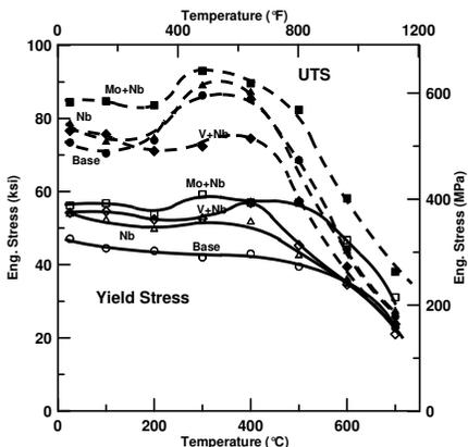
Figure 2. Yield stress (open symbols) and tensile stress (closed symbols) at 25°C – 700°C for Base, Nb, Mo+Nb, and V+Nb alloys, tested at an engineering strain rate of  $3.9 \times 10^{-3} \text{ s}^{-1}$  [19].
