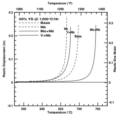
Figure 5. Constant loads test results for the Base, Nb, Mo+Nb, and V+Nb alloys at 50% yield strength for each alloy and 1200°C/hr [19].
