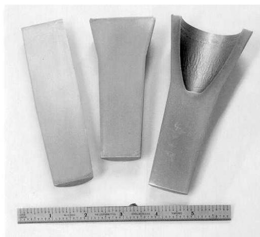
Figure 2: Forged C103 Bar to Nozzle Shape.
