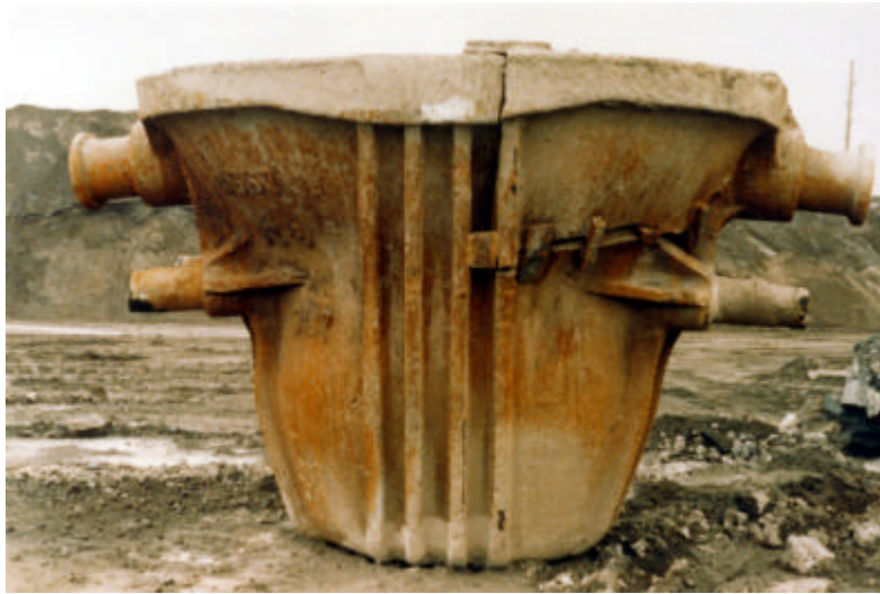
Figure 14: Conventional C-Mn steel slag pot showing “coke bottling” and fracture. Cast microalloyed slag pots exhibit a significant improvement in life (27). Courtesy of Johnstown Corporation, Johnstown, Pennsylvania, USA.
