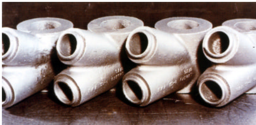
Figure 6: Machinery parts from 0.04% Nb-0.06% V steel (20). Courtesy of Thyssen Giesserei AG.
