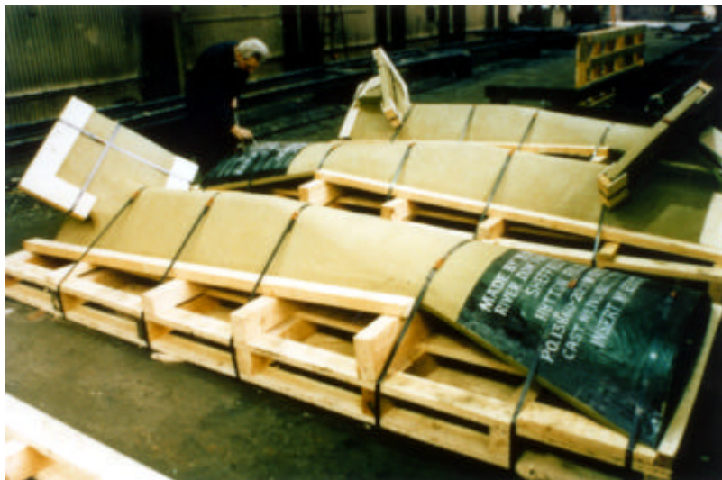
Figure 11: Insert castings for Conoco's Hutton tension-leg platform cast from Mo-Nb-V steel. Courtesy of River Don Castings, a member of Sheffield Forgemasters, Sheffield, England.
