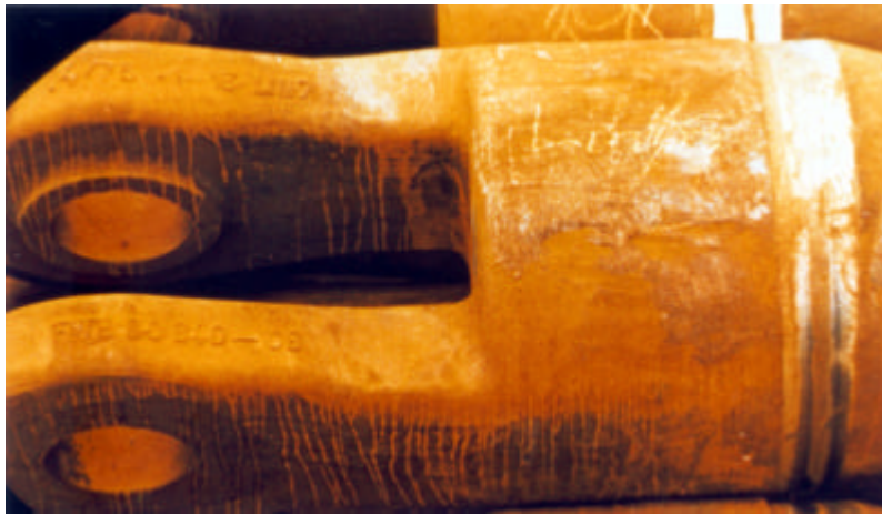
Figure 5: Connecting part weighing 665 kg (1465 lb) cast from 0.40% Mo-0.04% Nb-0.06% V steel for the supporting frame of a nuclear reactor (20). Courtesy of Thyssen Giesserei AG.
