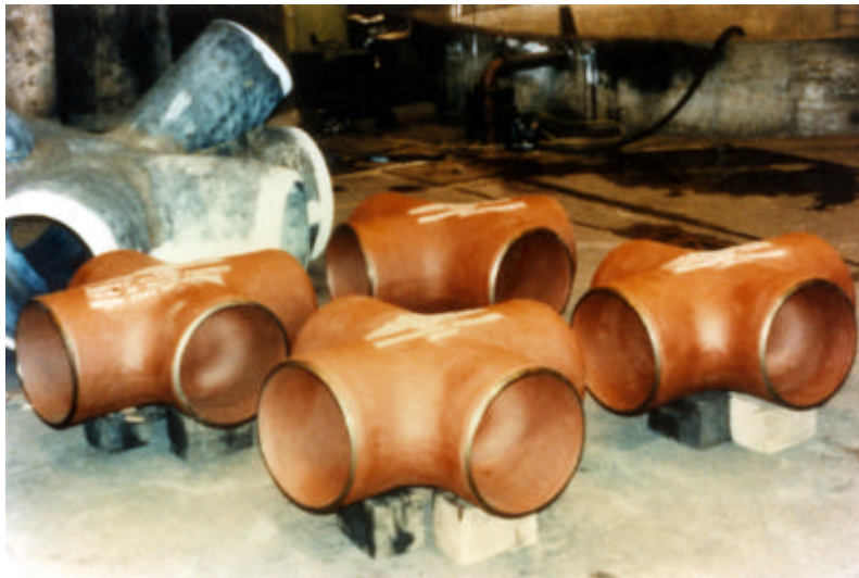
Figure 9: Niobium-containing cast steel nodes of offshore platform construction. Courtesy of River Don Castings, a member of Sheffield Forgemasters, Sheffield, England.
