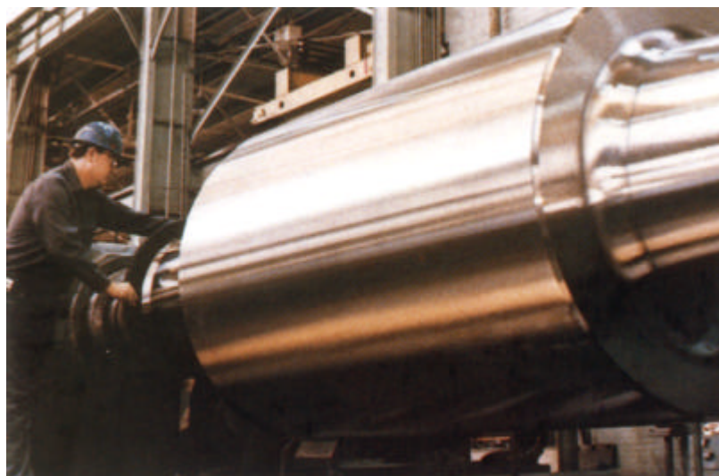
Figure 17: Cast steel back-up roll for hot-strip mill, grain refined using a 0.10% Nb addition (30). Courtesy of Blaw Knox Rolls, Wheeling, WV, USA.
