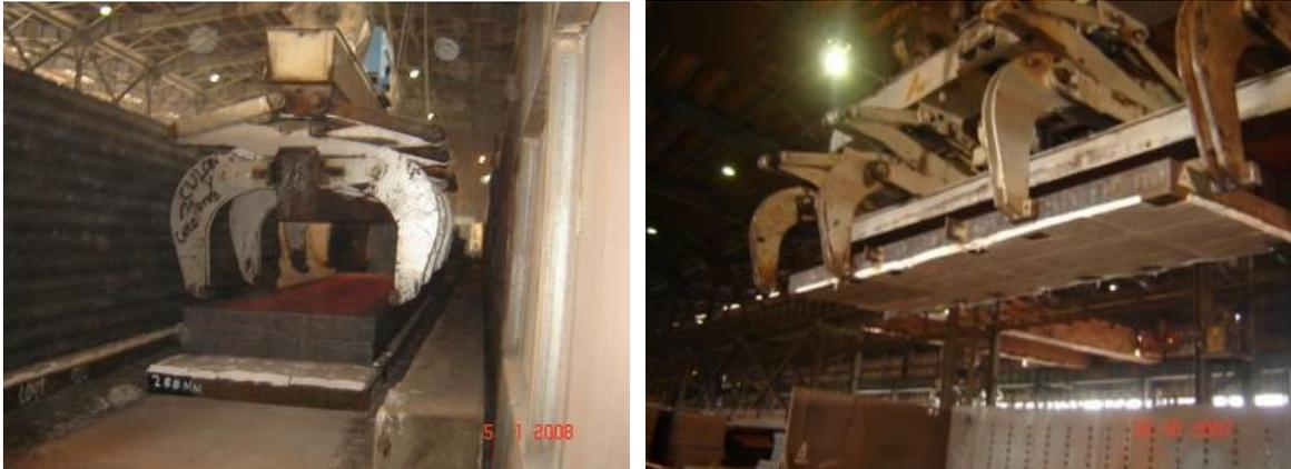
Figure 4. Controlled slow cooling of slabs for hydrogen removal.
