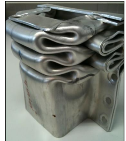
Crash samples: Ac-300 T61 2.5mm gauge, R_p \sim 220\text{MPa}
