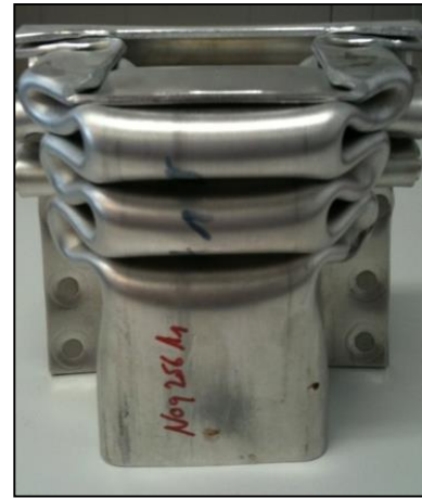
Crash samples: Ac-300 T61 2.5mm gauge, R_p \sim 220\text{MPa}
