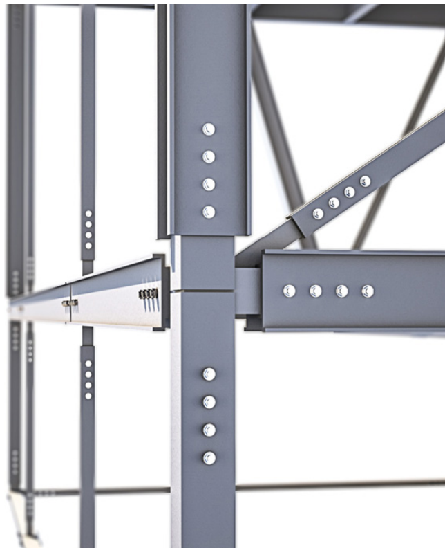
Fig. 6 – Support structure of the escalator with unrestrained column at the bottom and schematic detailing the typical bolted connections. Courtesy: Andrade Morettin Arquitetos Associados.
