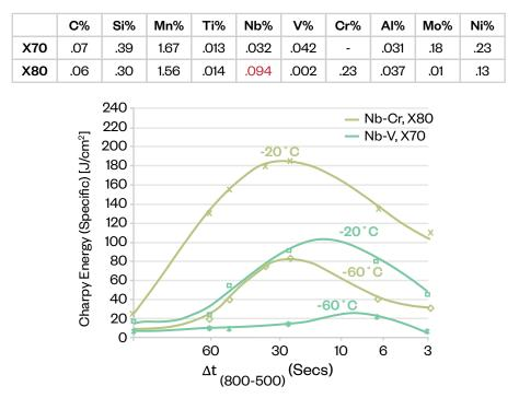
The effect of using a higher niobium content on the CGHAZ Charpy Toughness at different test temperatures and different cooling rates.
