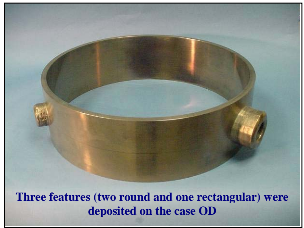
Figure 12: Images of Pratt & Whitney case that was fabricated from two 3" tall AMS 5662 rings EB welded together and machined to the nominal wall thickness of 0.5".
