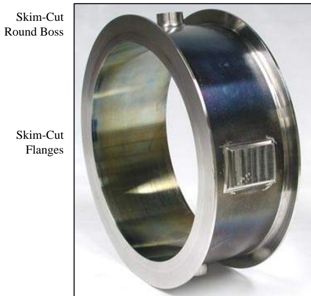
Figure 23: Photograph of EBWD deposited features on Rolls-Royce case section.
