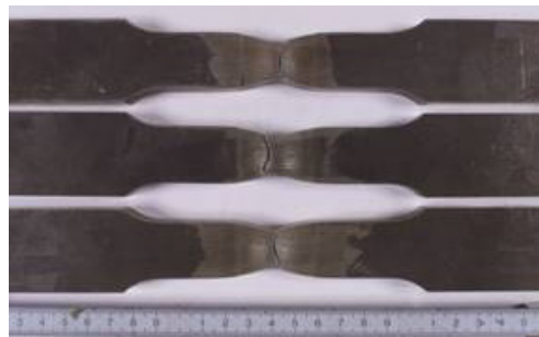
Figure 4. Fractured appearances of tensile test specimens
