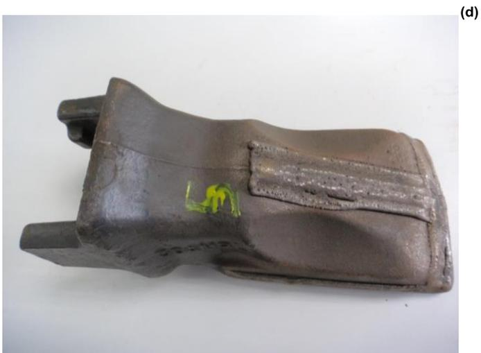
Figure 12. Volvo wheel loader steel tips coated with FeNbC; (a), (b) partial and (c), (d) total.
