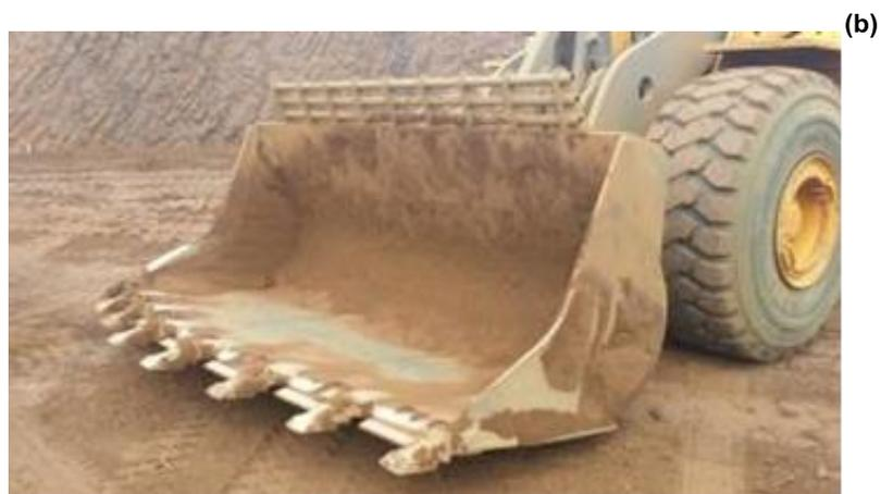
Figure 7. Assembling of the loader bucket teeth; (a) the four low alloy carbon steel tips coated with FeNbC are indicated with white arrows, (b) start of the field trials at CBMM's mine.
