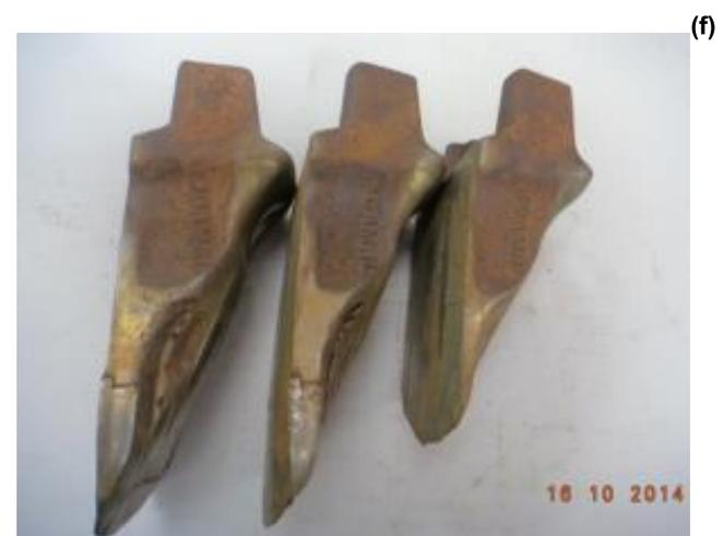
Figure 9. Wear patterns of the coated and uncoated teeth after the field trial. Top (a), (b), bottom (c), (d) and side (e), (f) views.
