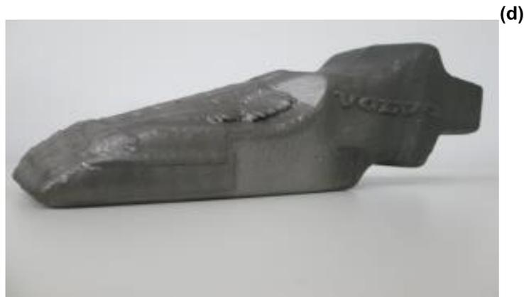
Figure 5. Volvo wheel loader steel teeth before (a) and after (b), (c) and (d) coating with FeNbC.
