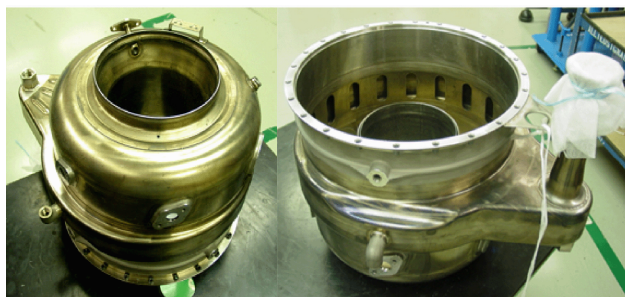
Figure 1. Honeywell GTCP36-150[BH] APU combustor plenum fabricated from Alloy 718 for U.S. Army, USAF, U.S. Navy and Coast Guard variants of the Sikorsky Blackhawk helicopter.
