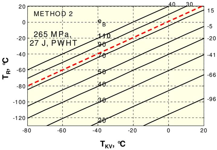
Figure 12a. New nomogram for conventional steel grades with strength level 265 MPa, dashed line allows use of thickness up to 110 mm if  $T_{KV} = 40$  J at  $T_R$ .
