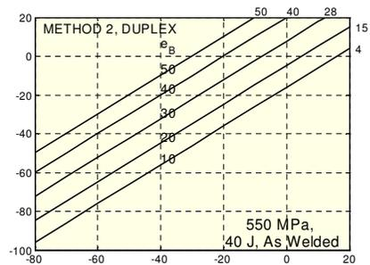
Figure 10b. Nomogram for austenitic ferritic  $Re \leq 550$  MPa.
