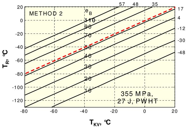
Figure 12b. New nomogram for conventional steel grades with strength level 355 MPa, dashed line allows use of thickness up to 110 mm if  $T_{KV} = 40$  J at  $T_R$ .
