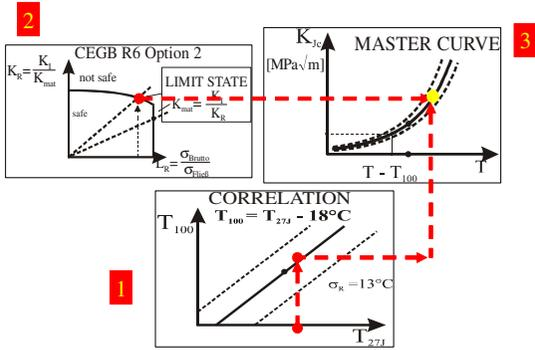
Figure 7. Principal derivation of limit state of fracture with fracture mechanics methods.
