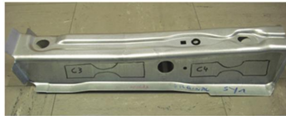
Figure 13. A-Pillar lower outside made from 2 mm CR330Y590T-DP (option W-2).
