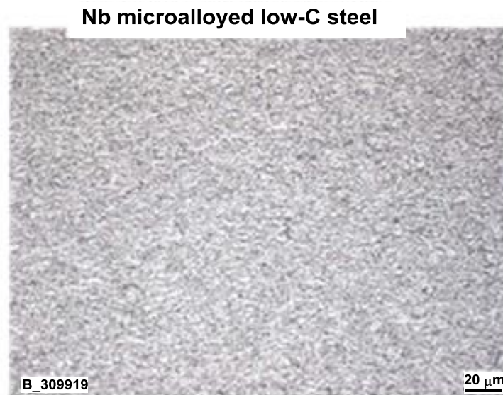
Figure 6. Effect of Nb microalloying on bainitic microstructure of low-C DP steel after coiling at 500 °C.
