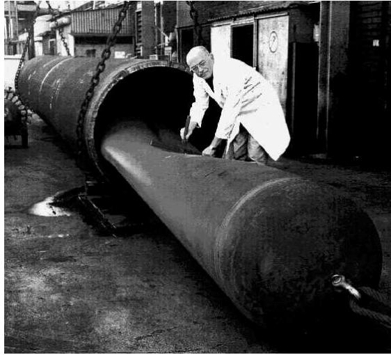
Figure 21: Photograph showing buckled linepipe section.
