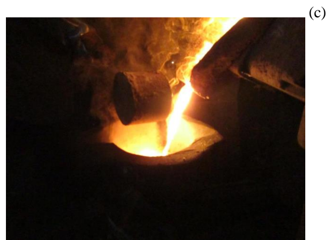
Figure 4. Methods of addition of FeNbC in iron castings: simple dumping on the surface (a), melting down with the charge (b) and addition to the metal stream during tapping (c).
