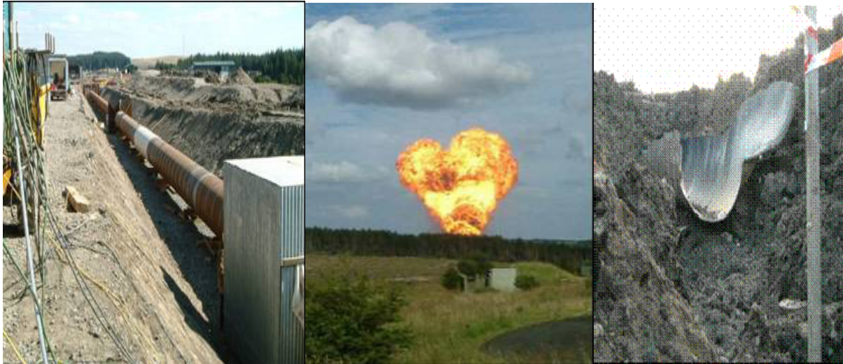
Figure 7. Construction of a fracture control test, detonation to initiate a running fracture and section of X100 pipe after test
