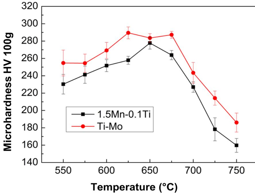
Figure 5. Effect of Mo on the microhardness of selected microstructures produced at different isothermal treatment temperatures.
