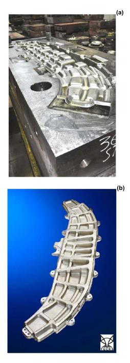
Figure 1. Example of a complex forging. (a) Die tool, (b) aluminum forging for an airplane [2].
