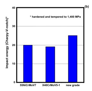
Figure 8. Yield strength and toughness of a new Nb microalloyed hot work steel in comparison to classical grades; (a) Yield strength, (b) Charpy toughness [12].
