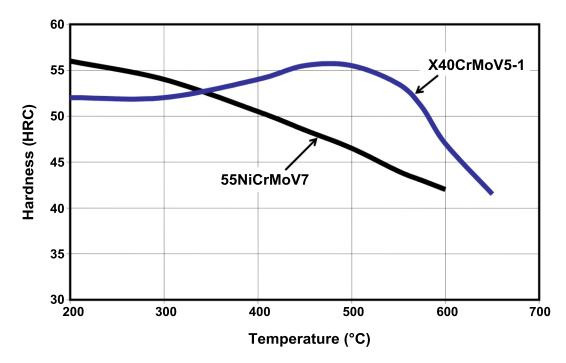
Figure 5. Tempering diagram of the hot work steels 55NiCrMoV7 and X40CrMoV5-1.
