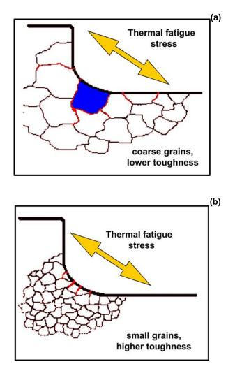
Figure 6. Effect of material toughness and grain size on thermal cracking of tools [6].
