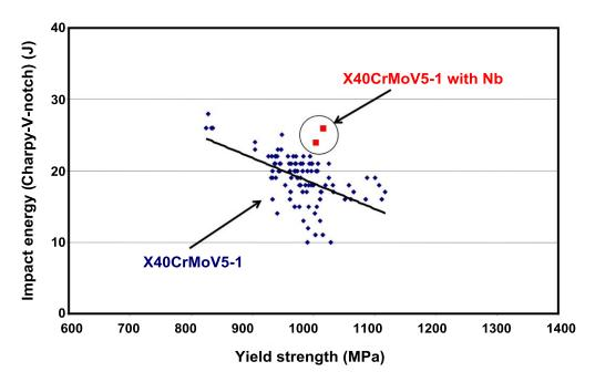
Figure 9. Results of mechanical testing steel bars in X40CrMoV5-1 for mandrels, toughness versus yield strength, in comparison with results for a Nb modified heat of the same grade.
