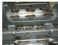
MIG-brazed: Crack in the parent material ! HC340X (DP-Steel) 1.0 mm + 1.0 mm
