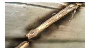
MIG-brazed: Crack in the parent material ! HC340X (DP-Steel) 1.0 mm + 1.0 mm
