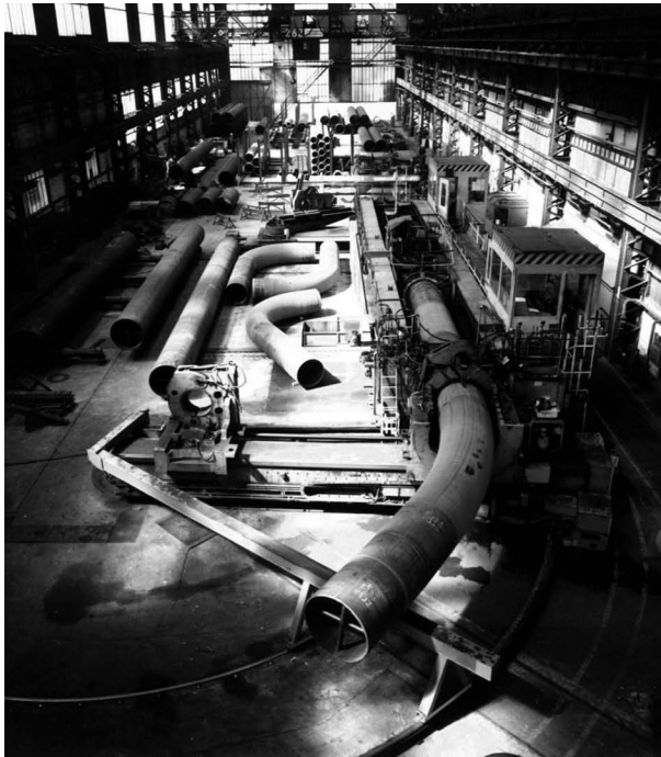
Figure 1. Hot induction bending of 48” line pipe @ Mannemann Bending Plant
