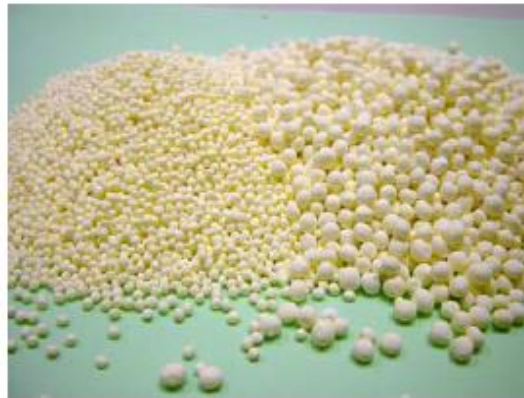
Figure 35. Ceramic beads used in ultrafine grinding.
