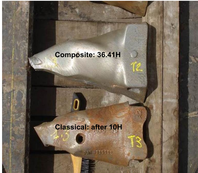
Figure 34. Xcc® dredging teeth compared to mono metal.
