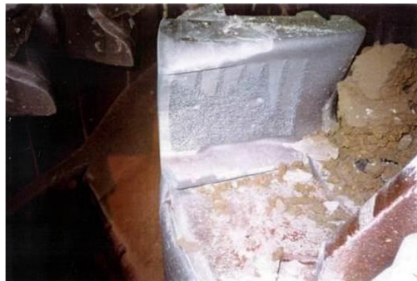
Figure 25. MMC impeller of VSI crusher.
