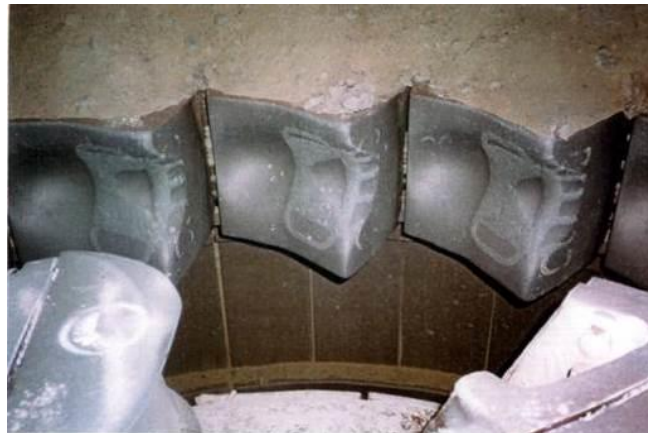
Figure 26. MMC anvil of VSI crusher.
