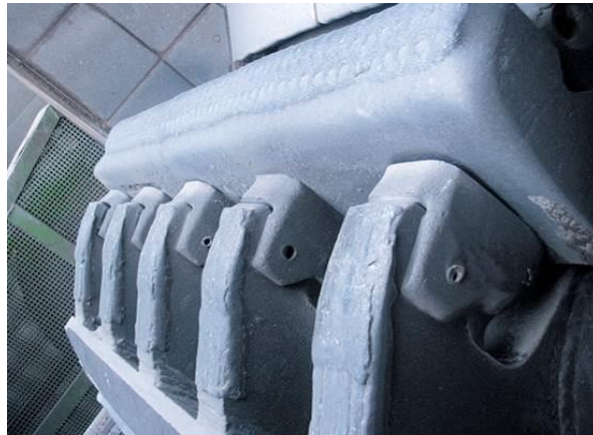
Figure 28. MMC blowbar of a horizontal shaft impact crusher.
