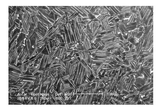
Figure 6 showing the convoluted microstructure formed in Ti46Al8Nb after oil quenching to room temperature and tempering the massively transformed sample at 1320°C for 1h.
