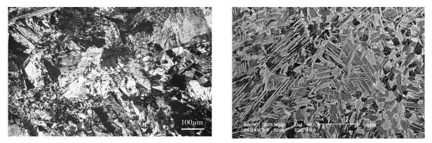
Figure 5. Backscattered scanning electron micrographs of Ti48Al2Nb2Cr showing in (a) the massively transformed structure in a sample air cooled from the alpha phase field and in (b) the convoluted microstructure formed on tempering the massively transformed structure for 2h at 1320°C. See text.
