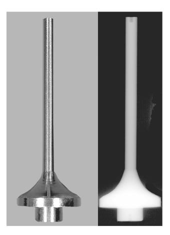
Figure 3 showing a roughly machined exhaust valve of Ti44Al8Nb1B and the corresponding X-ray radiograph, which does not reveal any porosity. Melting was carried out using a CaO crucible which allowed a superheat of 160°C, and the valve was cast using centrifugal casting into a pre-heated ceramic mould. (Courtesy IMR, Shenyang, China).
