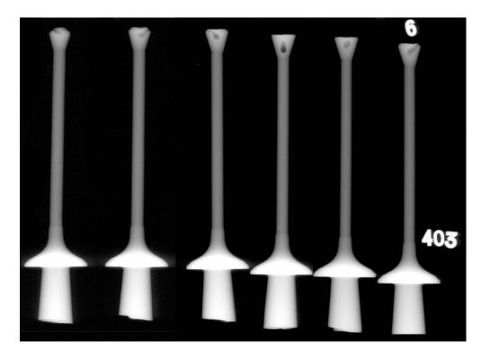
Figure 2 X-ray radiographsTi44Al8Nb1B valves cast using counter gravity casting showing no obvious pores. Compare figure 1. (Courtesy R A Harding).
