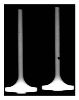
Figure 1 X-ray radiographs showing pores in valves of Ti48Al8Nb1B cast using a cold wall furnace to melt the alloy which was heated to about 50°C above its melting point before pouring into a ceramic mould pre-heated to 1000°C
