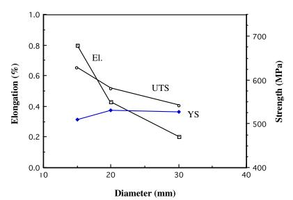
Figure 4 showing the influence of the diameter of cast bars of Ti44Al8Nb1B on the room temperature tensile properties.
