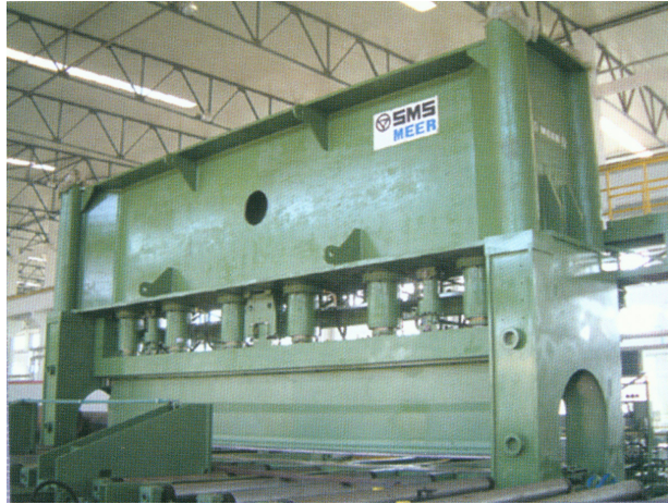
Figure. 13. The imported JCO forming machine for longitudinal saw pipe production in Julong ( Huabei ) Steel Pipe Co.
