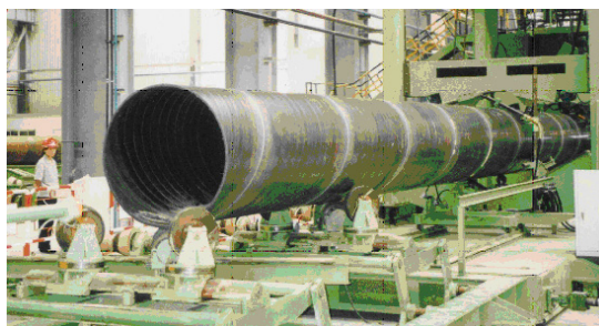
Figure 11. The domestically build new spiral welding pipe facility in BAOJI pipe mill.
