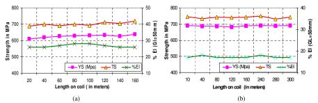
Figure 4. Tensile properties variation along the coil length a) grade SR60 and b) grade SR65.
