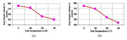
Figure 7. Impact energy transition curve for a) SR60 and b) SR65.
