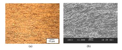
Figure 9. Photo-micrographs of SR65 a) Optical micro-photograph (Etchant: Le Pera) and b) Scanning Electron Micro-scope (Etchant: 2% Nital).
