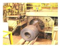
Figure 3. Steel coil after hot rolling at Hot Strip Mill, Essar
