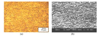
Figure 8. Photo-micrographs of SR60 a) Optical micro-photograph (Etchant: Le Pera) and b) Scanning Electron Micro-scope (Etchant: 2% Nital).
