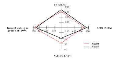
Figure 5. Comparison of typical mechanical properties of SR60 and SR65 grade steel.
