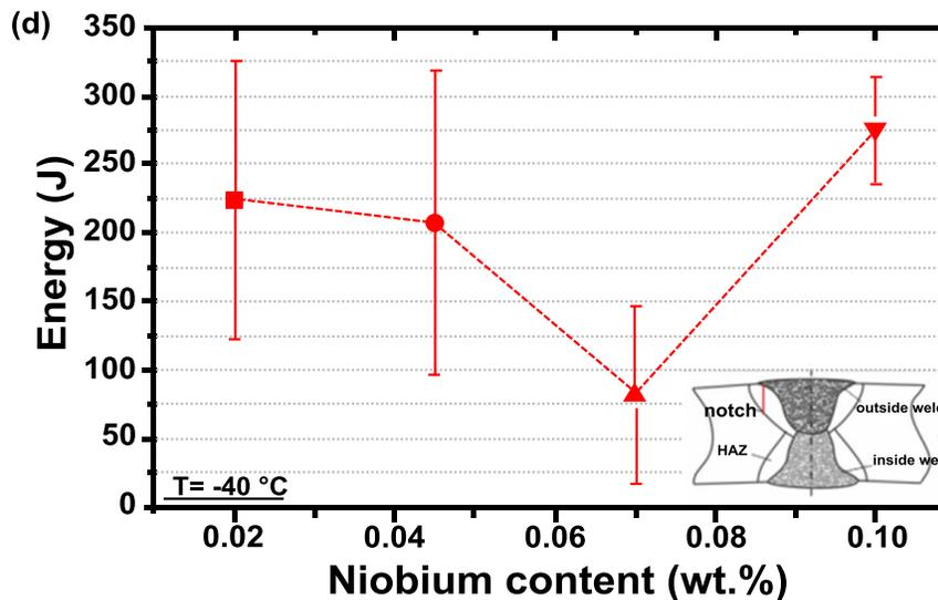
Figure 11. Evolution of Charpy impact energy depending on the Nb content for test temperatures; (a) -20 °C and (b) -40 °C, notch position according to DNV-OS-F101, as well as (c) -20 °C and (d) -40 °C, notch position according to ISO 3183.
