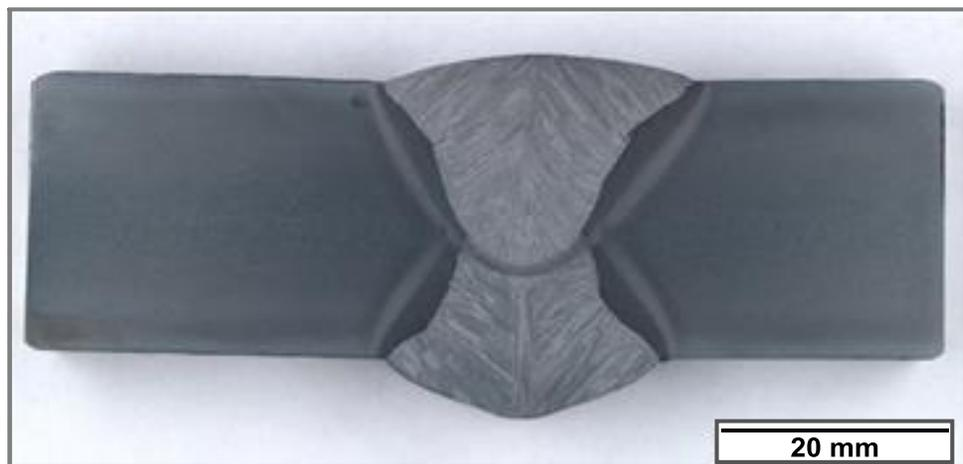
Figure 9. Cross section of SA weld, Nb content 0.022%.
