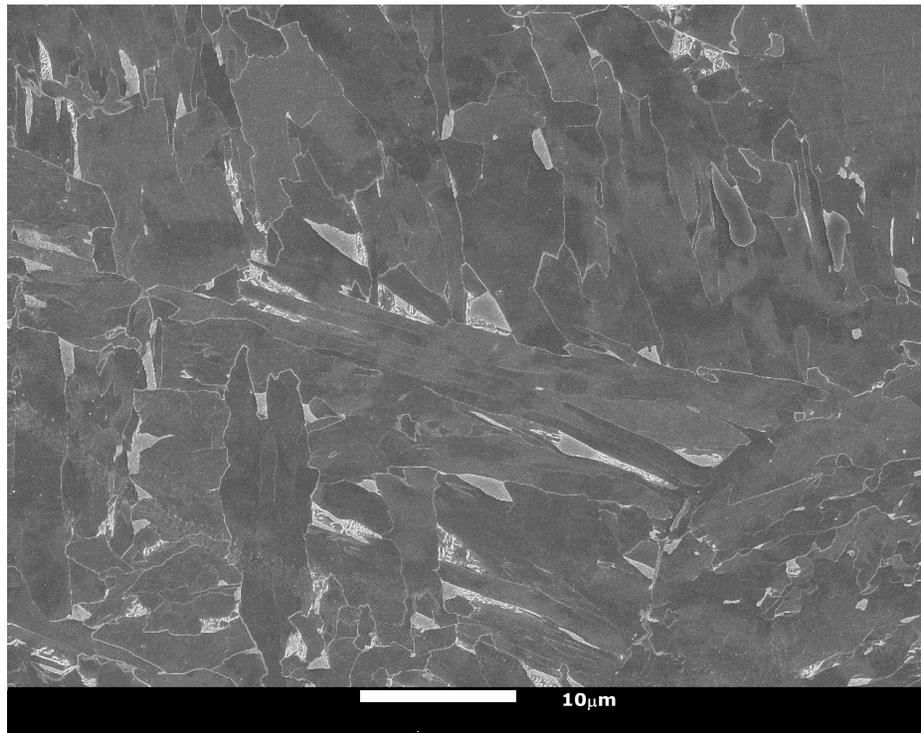
Figure 15. Example of the microstructure in the CGHAZ.
