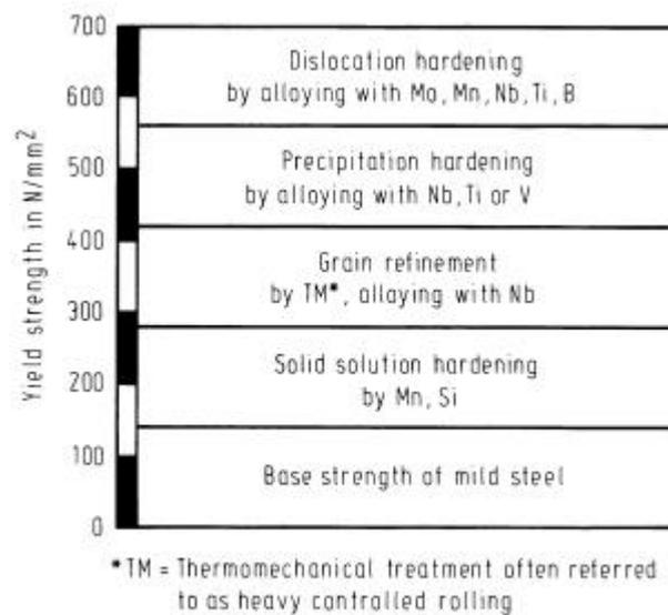
Figure 10: Contribution of various strengthening mechanisms via alloying and processing to achieve 700MPa yield strength in hot strip.
