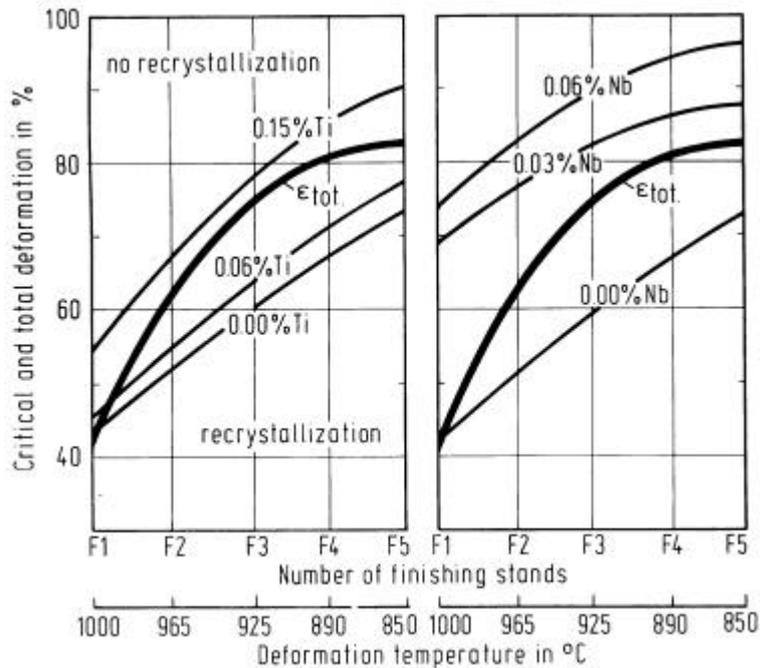
Figure 9: Critical deformation for dynamic recrystallization of Ti or Nb microalloyed steel compared to the total deformation in the finishing train of a hot strip mill.
