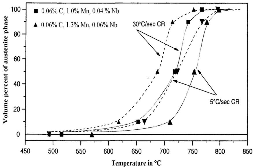
Figure 17: Phase transformation curve of two steels and two cooling rates (reheated to 1000°C and linearly cooled).
