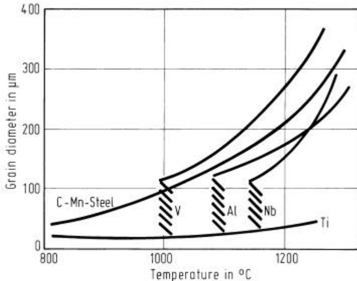
Figure 13: Austenite grain growth characteristics in steels containing various microalloy additions.
