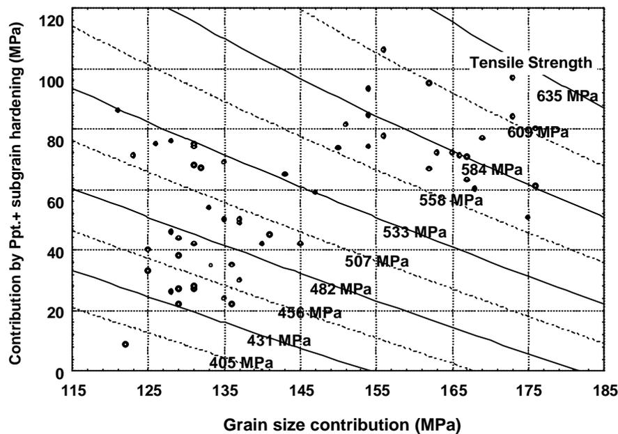
Figure 25: Contribution of various strengthening mechanisms on the strength of HSLA strip (0.055-0.075 %C, 0.4-1.5 %Mn, 0.02-0.06 % Nb).
