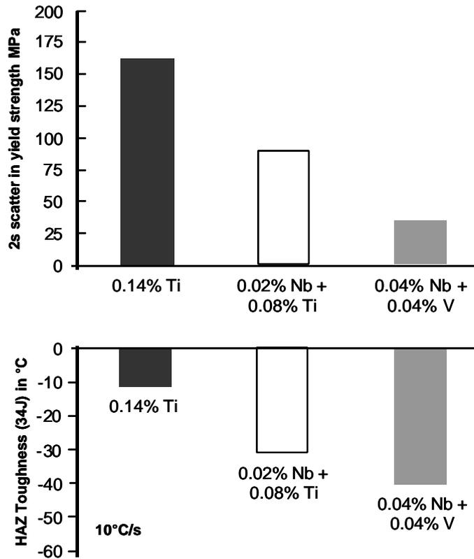
Figure 8: Different microalloy concepts in the production of HSLA strip Grade 70 ( $R_{e \min}=500\text{MPa}$ ) and resulting properties with regard to scatter in yield strength and toughness in the heat-affected zone. Base composition: 0.07%C, 1.10%Mn.
