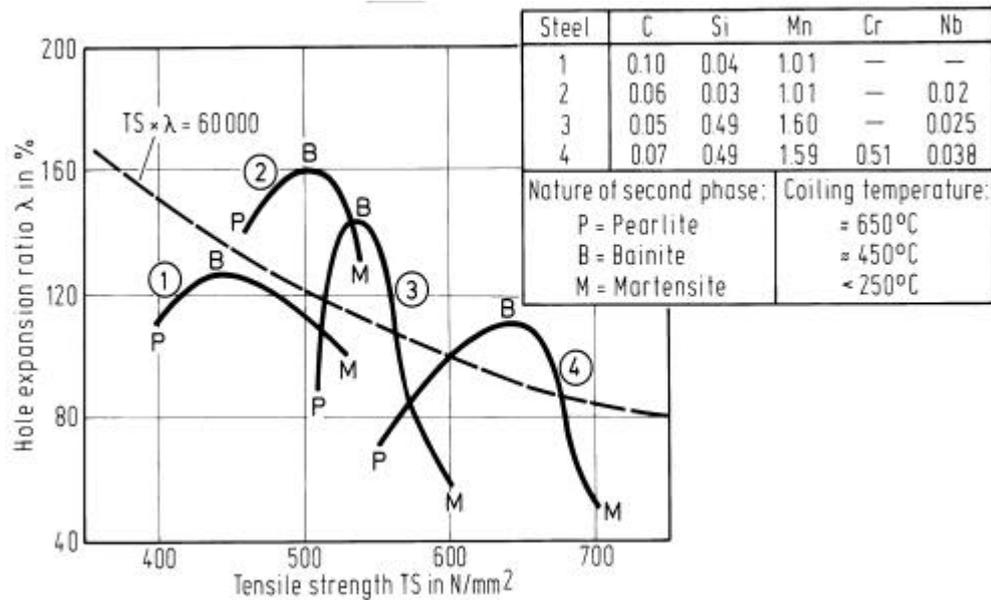
Figure 20: Influence of coiling temperature and alloy design on the microstructure and properties of HSLA strip.
