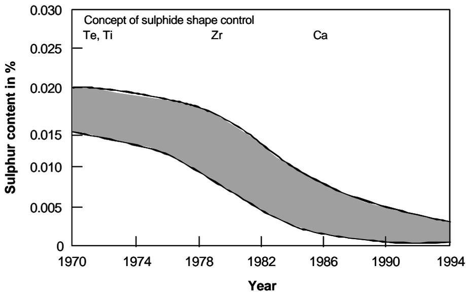
Figure 5: Sulphur concepts for HSLA strip in the last decades.
