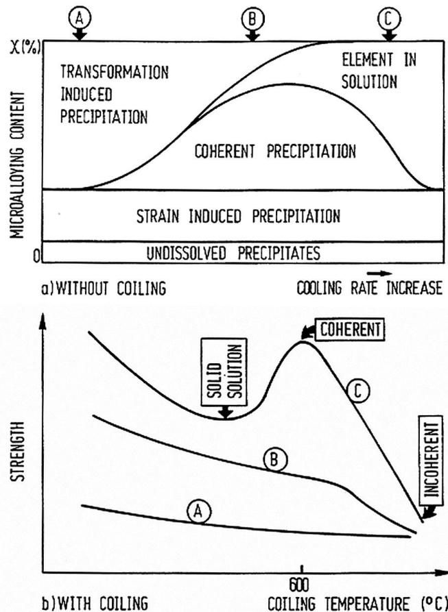
Figure 16: Influence of processing conditions on the nature of precipitates and the resulting strength – schematically.
