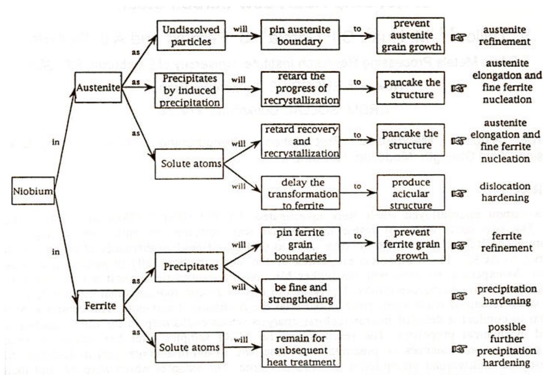
Figure 23: Schematics of the different roles of niobium during thermomechanical rolling.
