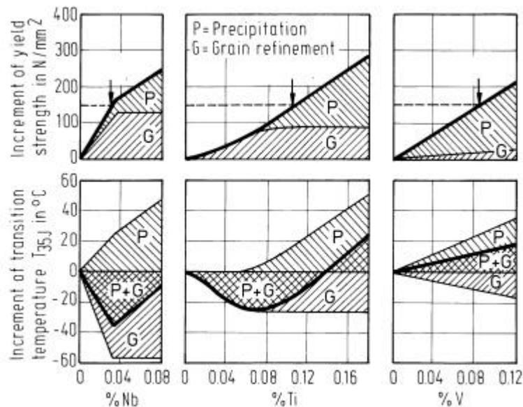
Figure 7: The effect of microalloy additions to the properties of mild hot strip steel.
