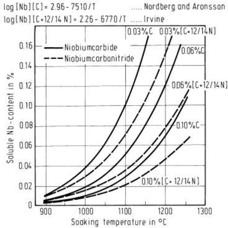
Figure 12: Solubility of niobium carbides and carbonitrides in low carbon steel.
