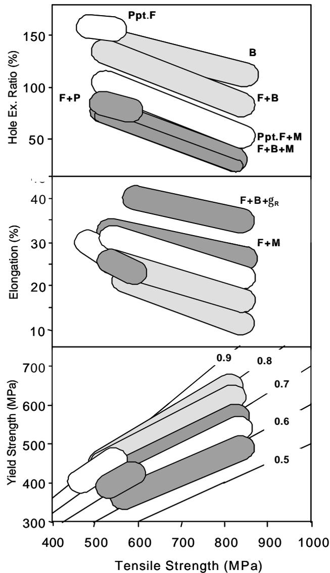
Figure 2: Relationship between microstructure and properties. Key: F = ferrite; P = pearlite; B = bainite; M = martensite;  $a_R$  = retained austenite; ppt = precipitates.
