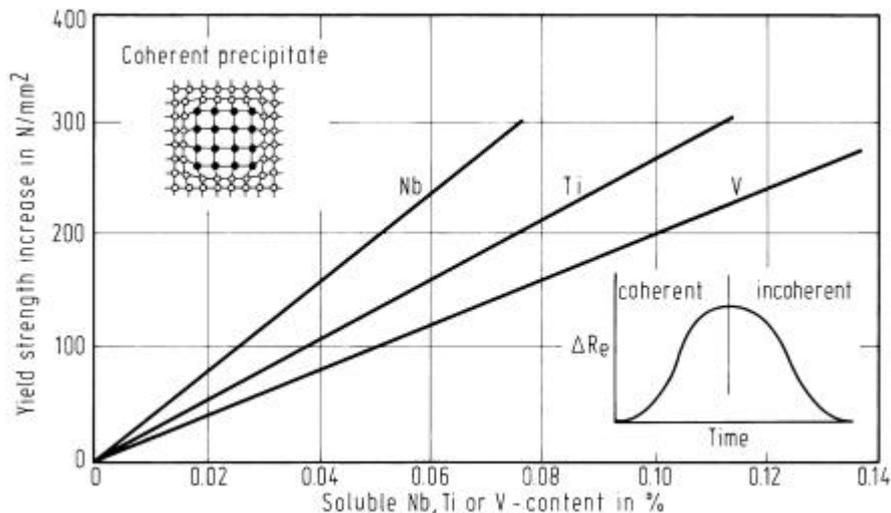
Figure 18: Maximum yield strength increase by precipitation hardening for a wide range of steel compositions, solution treated at 1300°C and isothermal holding at 600°C.
