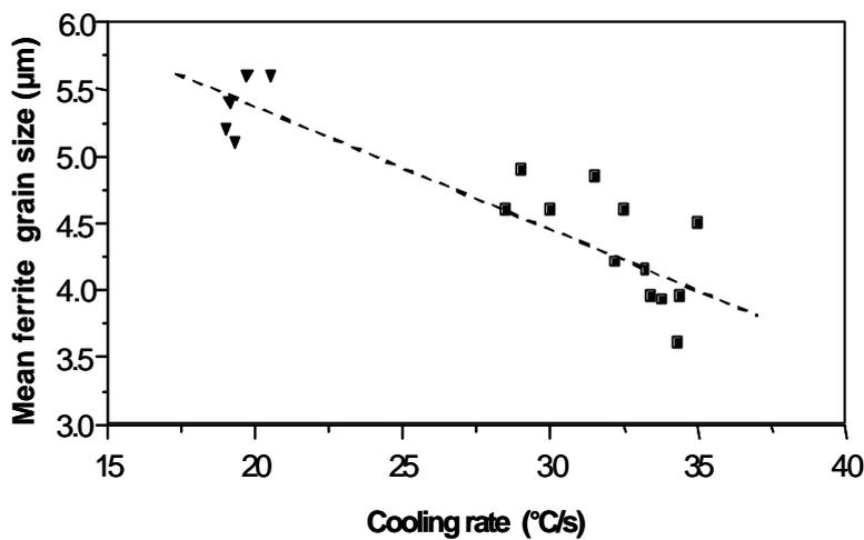
Figure 14: Influence of cooling rate in the run-out table on the ferrite grain size of HSLA strip.
