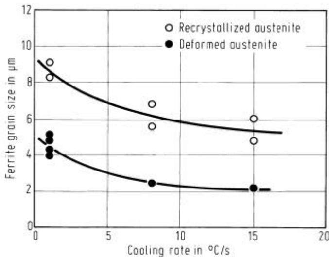
Figure 15: The effect of austenite processing and cooling rate on the final ferrite grain size.
