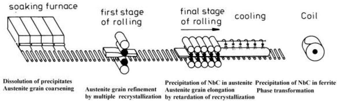
Figure 11: Metallurgical processes during hot strip rolling of HSLA steel.
