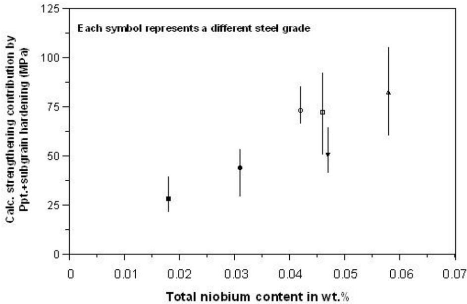
Figure 24: Relationship between niobium content and strength increase by precipitation and subgrain hardening.
