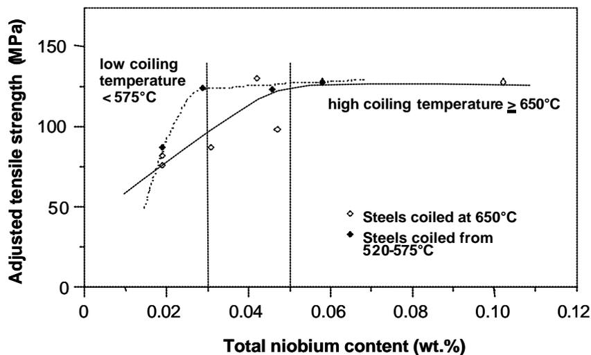
Figure 19: Adjusted tensile strength as result of the niobium content and coiling temperature.
