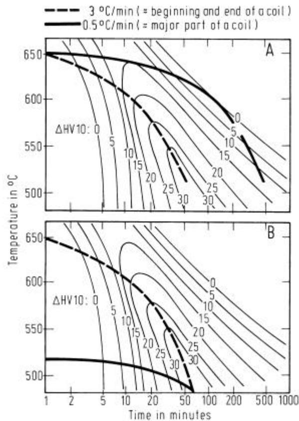
Figure 22: Iso-hardness curves as result of precipitation hardening by NbC of steel with 0.02% solute niobium with the cooling curves for different coil positions superimposed. a) Constant coiling temperature; b): Maximum and homogeneous strength.
