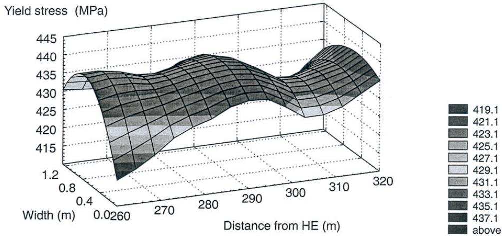
Figure 21: Topological yield strength distribution for a niobium HSLA strip.
