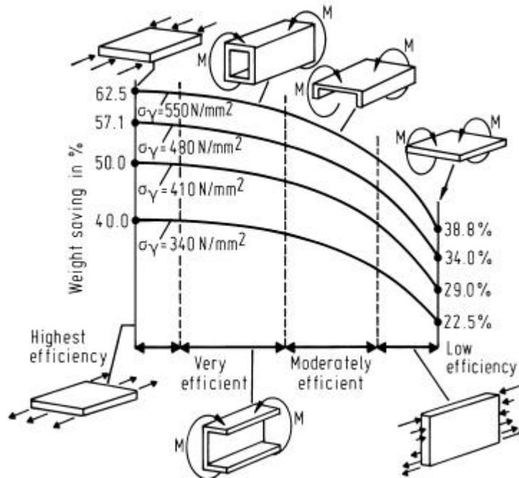
Figure 3: Potential weight savings when substituting a 200MPa yield strength steel.
