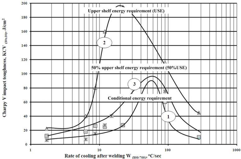
Figure 9. Determination of allowable cooling rate for maintenance of adequate HAZ impact toughness at -30 °C for steels 1, 2 and 3 depending on energy requirement (USE, 50% or conditional).
