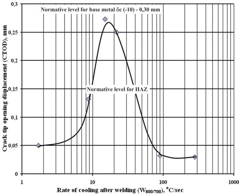
Figure 10. Influence of cooling rate on change of CTOD value, steel N° 3.
