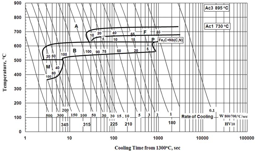
Figure 3. Austenite transformation diagram for the HAZ of steel N° 2.
