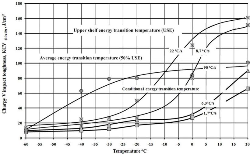
Figure 5. HAZ transition curves for different cooling rates, steel N<sup>o</sup> 1.
