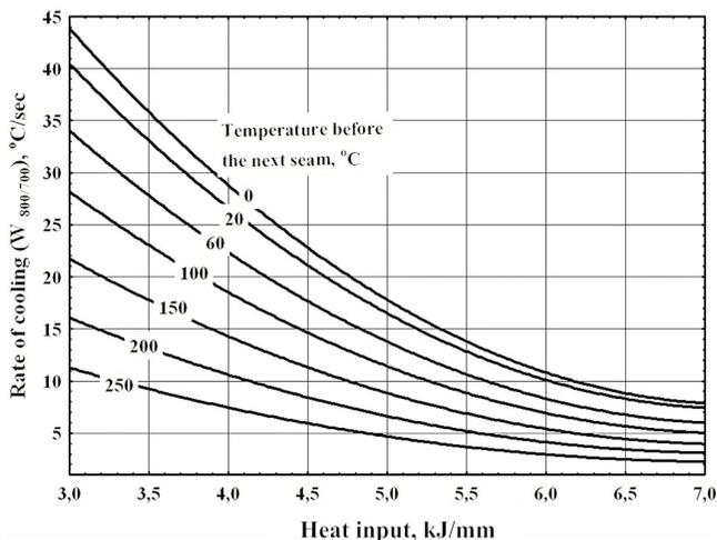
Figure 1. Determination of cooling rate after welding (pipes with thickness 25.4 mm) from heat input and temperatures before welding ( $W_{800/700} = 1,92 \times W_{800/500}$ ).
