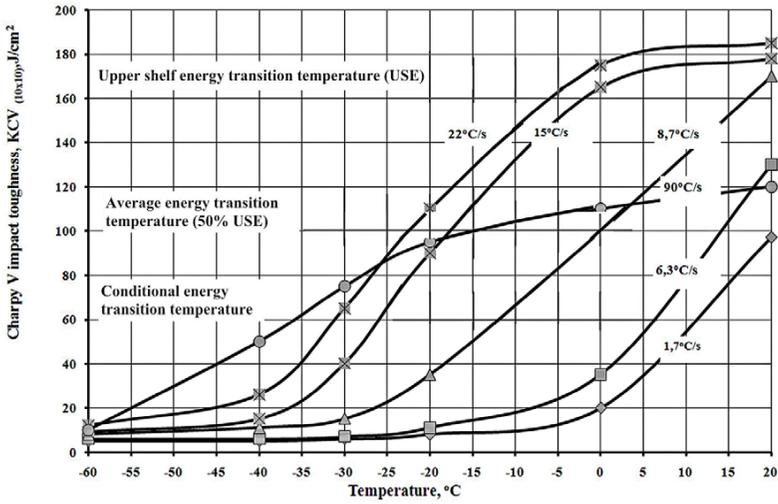
Figure 7. HAZ Charpy transition curves for different cooling rates, steel N° 3.
