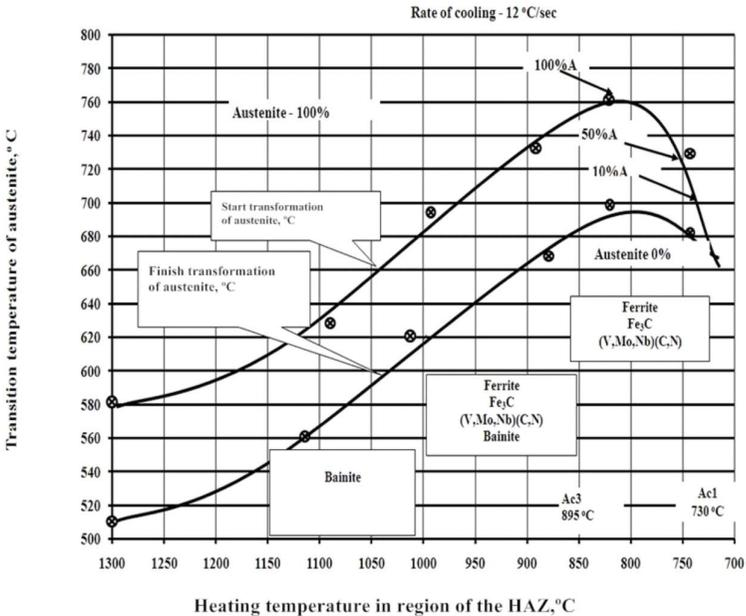
Figure 4. Change of austenite transformation temperature in the HAZ after heating to 1300 to 730 °C.
