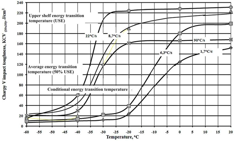
Figure 6. HAZ Charpy transition curves for different cooling rates, steel N° 2.
