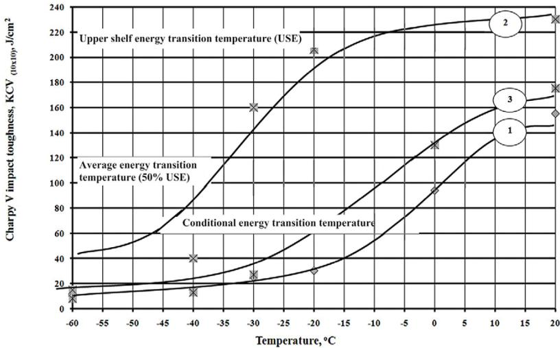
Figure 8. Comparison of HAZ Charpy transition curves for a cooling rate of 12 °C/s for steels 1, 2 and 3.
