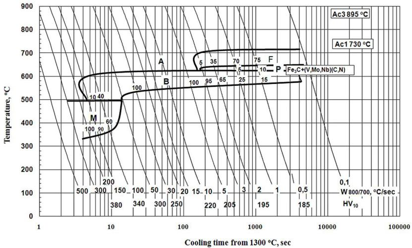
Figure 2. Austenite transformation diagram for the HAZ of steel N° 1.
