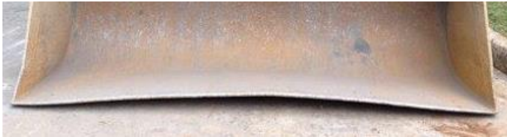
Figure 2. Bucket deformation after 200 hours in service.
