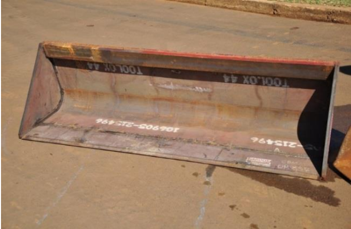
Figure 15. New bucket design after 1,650 hours of work time. No cracks and no deformation.
