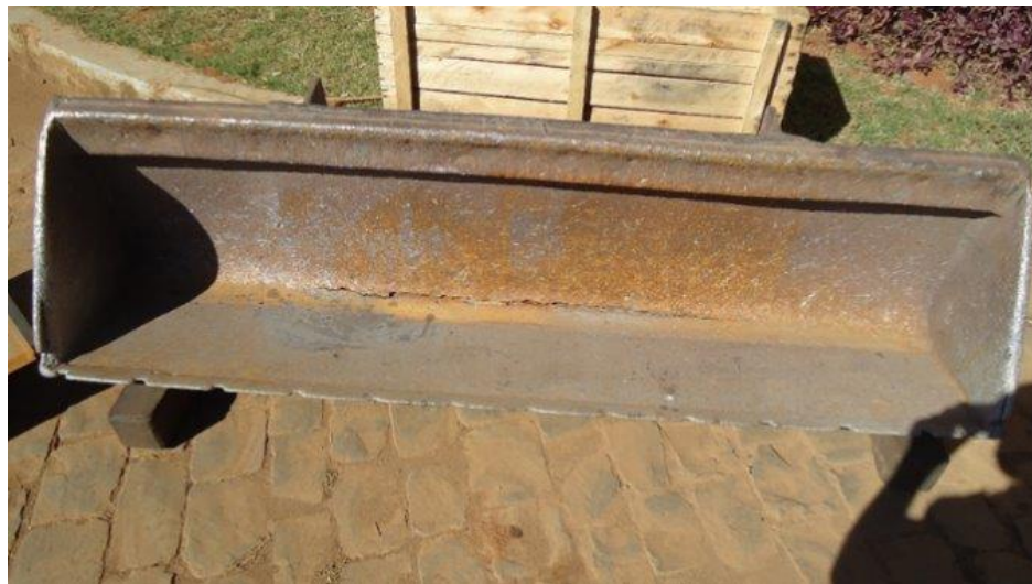
Figure 3. Bucket cracking after 200 hours in service.
