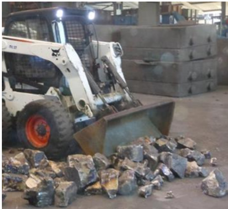
Figure 1. Loader collecting FeNb after ingot stripping.
