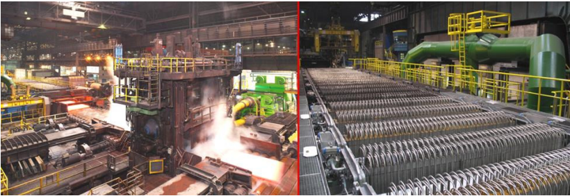
Figure 1. 4.2m wide plate rolling mill and cooling line at voestalpine Grobblech GmbH.
