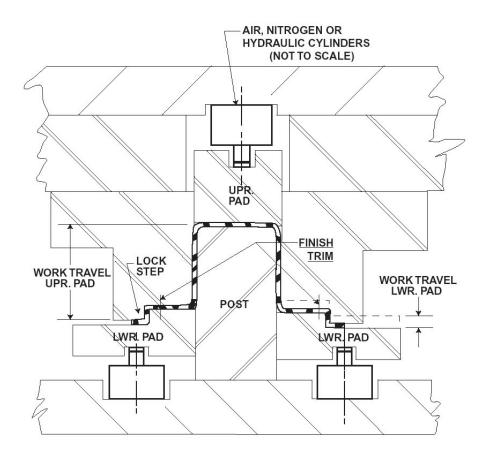
Figure 4. Post stretch form die with lower pad to enhance sidewall stretch (from Auto/Steel Partnership High Strength Steel Design Manual) [21].
