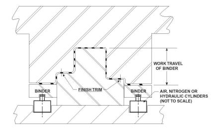
Figure 5. Draw die in single action press. An upper pad (not shown) is often used to control part shape (from Auto/Steel Partnership High Strength Steel Design Manual) [21].
