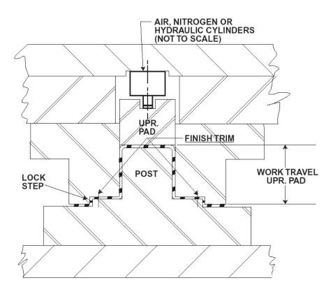
Figure 3. Post stretch form die - showing lock step which helps stretch sidewalls (from Auto/Steel Partnership High Strength Steel Design Manual) [21].
