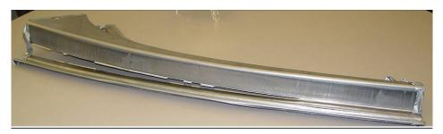
Figure 2. DP800 stamping exhibiting shear fracture.
