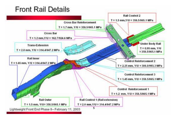
Figure 1. Front rail design from Auto Steel Partnership Lightweight Front End Structure Project – All components are Dual Phase steel. Target mechanical properties shown.
