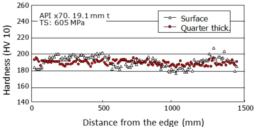
Figure 18. Hardness distributions across the width of X70 sour linepipe steel plate.
