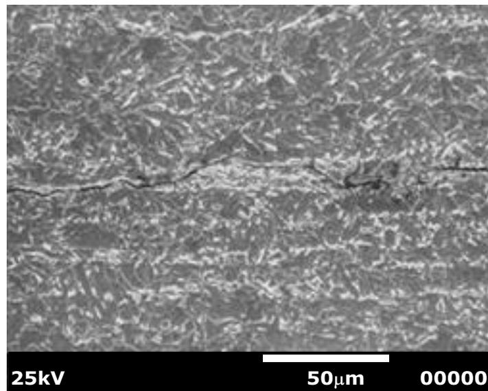
Figure 2. Cracking in the center segregation zone.
