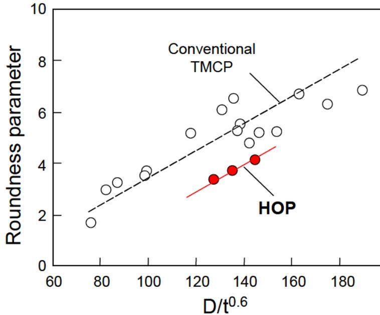
Figure 21. Relationship between roundness and  $D/t^{0.6}$  for linepipes with different manufacturing processes.
