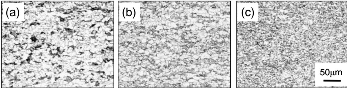
Figure 4. Microstructure of X65 linepipe accelerated cooled from different temperatures; (a) 760 °C, (b) 730 °C and (c) 690 °C.
