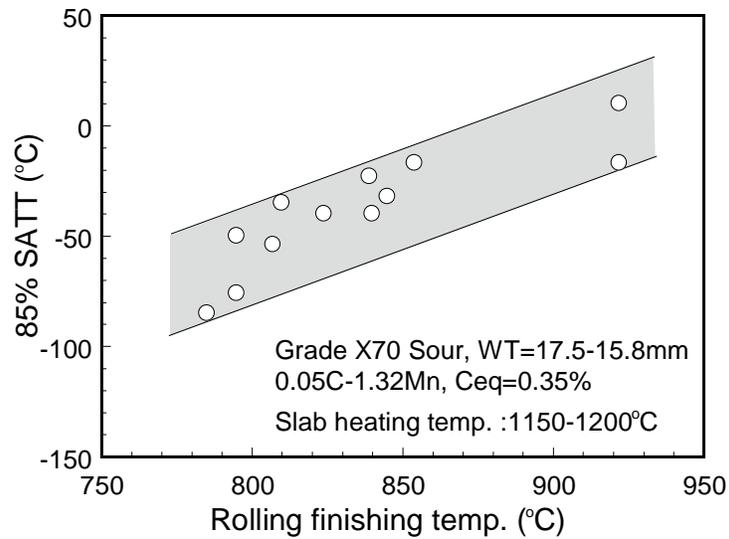
Figure 11. Relationship between DWTT shear area transition temperature and finish-rolling temperature.
