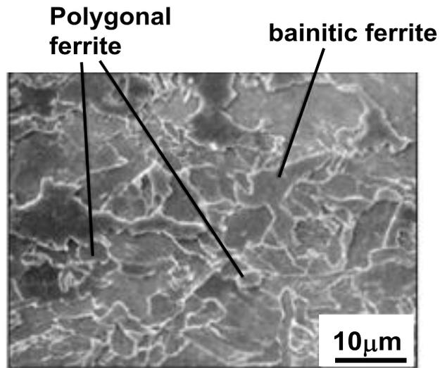
Figure 19. SEM micrograph of X70 sour linepipe produced by the HOP process.
