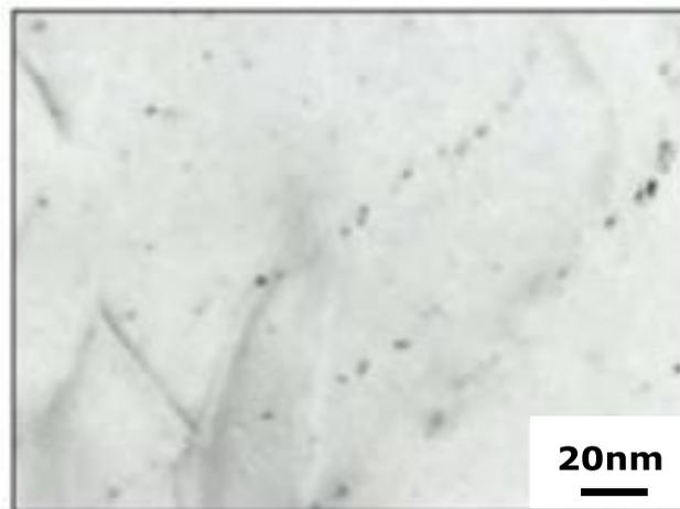
Figure 20. TEM micrograph of X70 sour linepipe produced by the HOP process.
