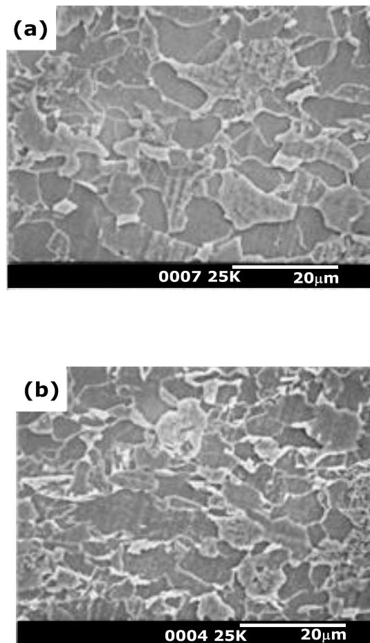
Figure 8. SEM micrographs of the plates accelerated cooled with cooling rates of; (a) 10 °C/s and (b) 30 °C/s.
