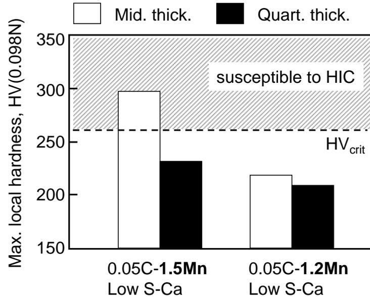
Figure 3. Effect of Mn content on maximum local zone hardness.
