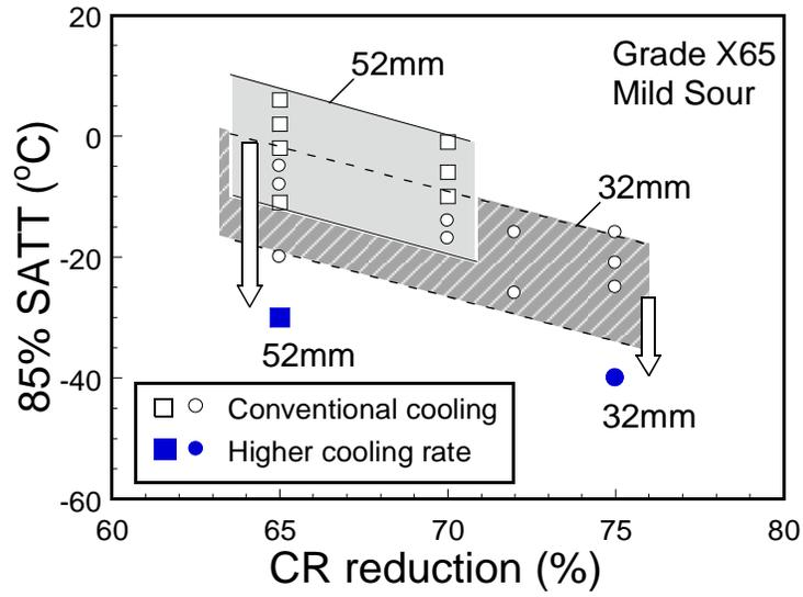
Figure 10. Relationship between DWTT shear area transition temperature and reduction in controlled rolling.
