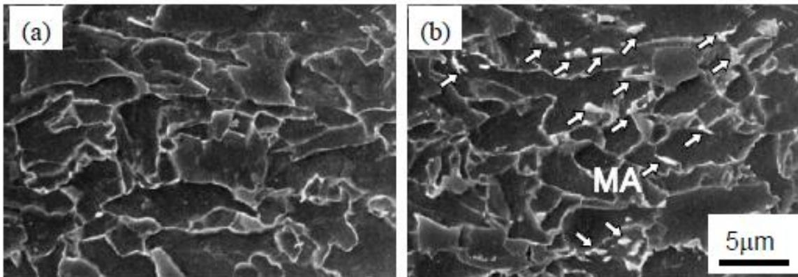
Figure 15. SEM micrographs of the steels etched by two-stage electrolytic etching;
