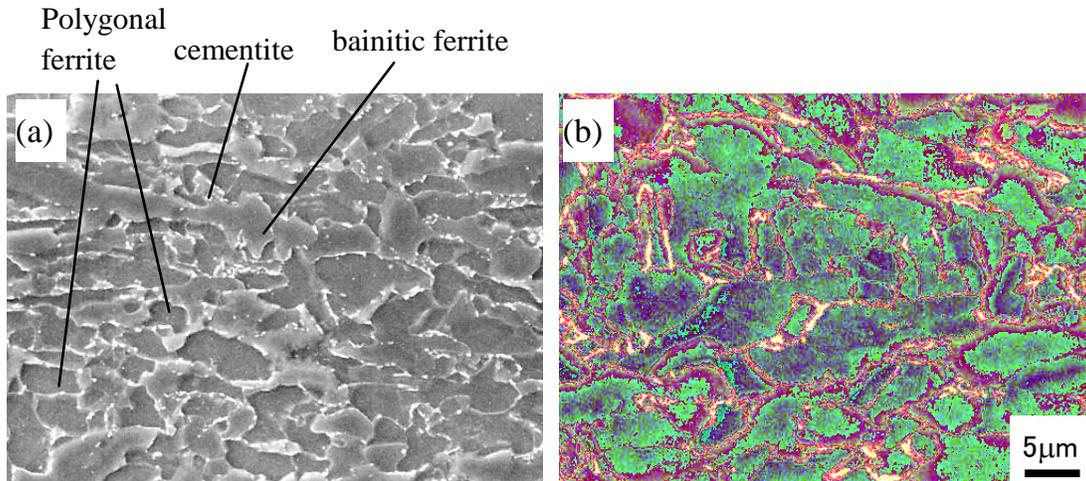
Figure 14. SEM micrographs of the steels etched in 3% Nital;
