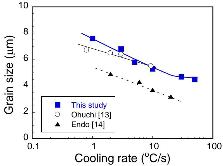
Figure 7. Effect of cooling rate on grain size of accelerated cooled plates.
