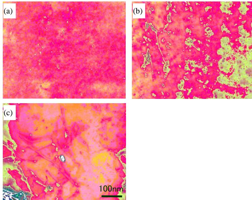
Figure 16. TEM micrographs of the steels; (a) HOP, random precipitates, (b) HOP, precipitate rows, (c) conventional TMCP, relatively large precipitates.
