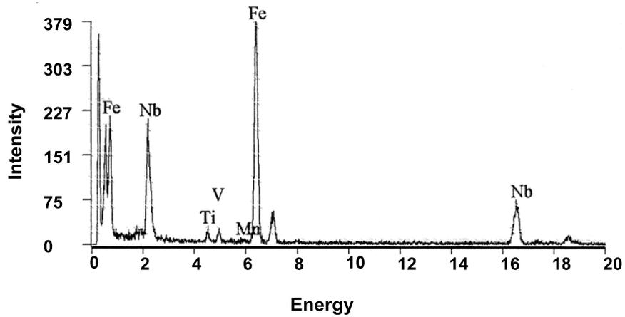
Figure 17. EDS spectrum of the precipitates.
