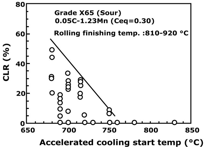
Figure 5. Relationship between accelerated cooling start temperature and CLR.
