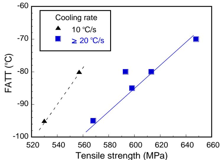
Figure 6. Relationship between tensile strength and Charpy impact toughness (FATT) of the steel plates accelerated cooled with different cooling rates.
