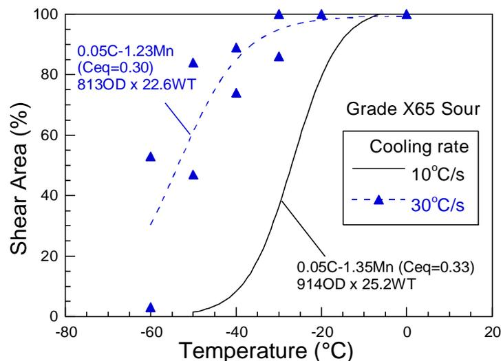
Figure 9. DWTT shear area transition curves of Grade X65 linepipes produced with different cooling rates in accelerated cooling process.
