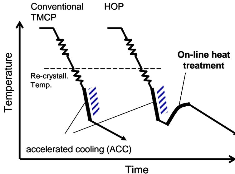
Figure 12. Schematic temperature profiles in plate production process.
