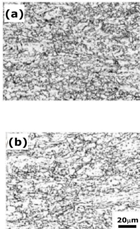
Figure 13. Optical micrographs of the steels etched in 3% Nital; (a) HOP process, (b) conventional TMCP.
