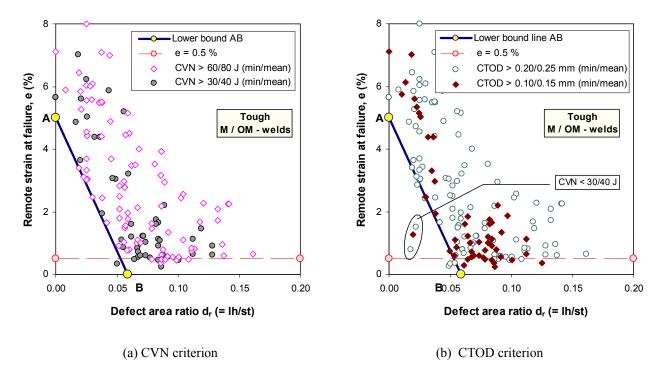
Figure 2. Variation of overall remote strain, e, with defect area ratio, d<sub>r</sub>, in overmatched welds as a function of CVN or CTOD toughness (see insert to the plots).
