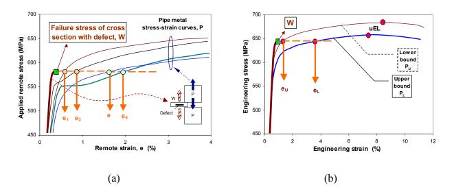
Figure 6. Effect of strain hardening behaviour on remote strain
