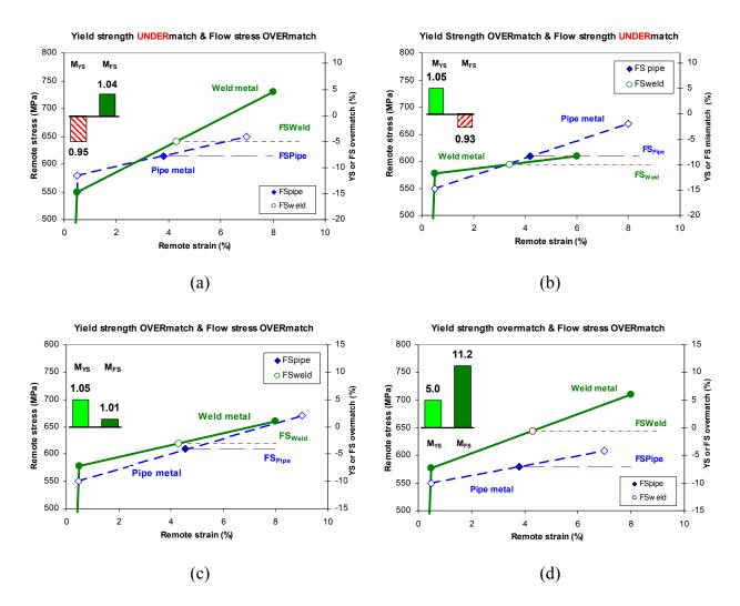
Figure 8. Effect of post-yield stress-strain behaviour on strength mismatch
