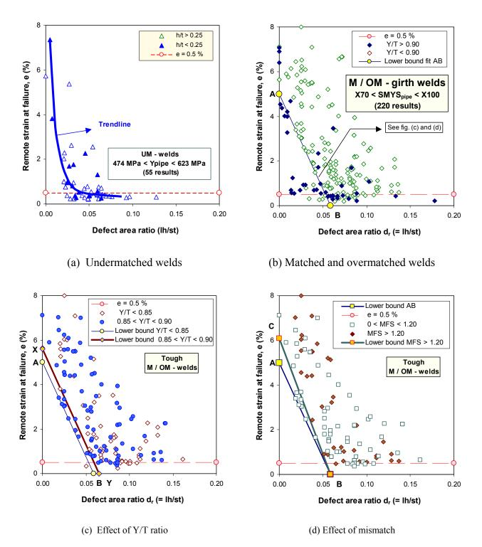
Figure 1. Variation of remote failure strain as a function of defect area ratio (lh/st) for (a) undermatched, (b)(c) and (d) matched and overmatched girth welds. Data in (c) and (d) showresults of tough girth welds as a function of pipe metal Y/T ratio and strength mismatch (see key).
