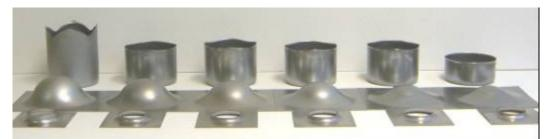
Figure 6. Results from deep drawing tests (rear), stretch forming tests (center) and hole expansion tests (front) of various steel grades (rom left to right): DC04, Docol 600 DL, Docol 600 DP, Docol 800 DP, Docol 1000 DP and Docol 1400 M.
