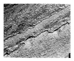
Figure 9: Surface Tears Preform ~ 13X.
