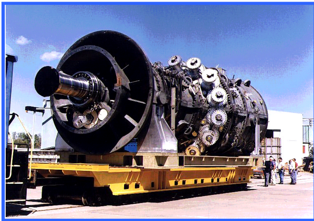
Figure 14: First MS9001H gas turbine at GE's facilities (Greenville, SC). Courtesy of General Electric Power Systems.
