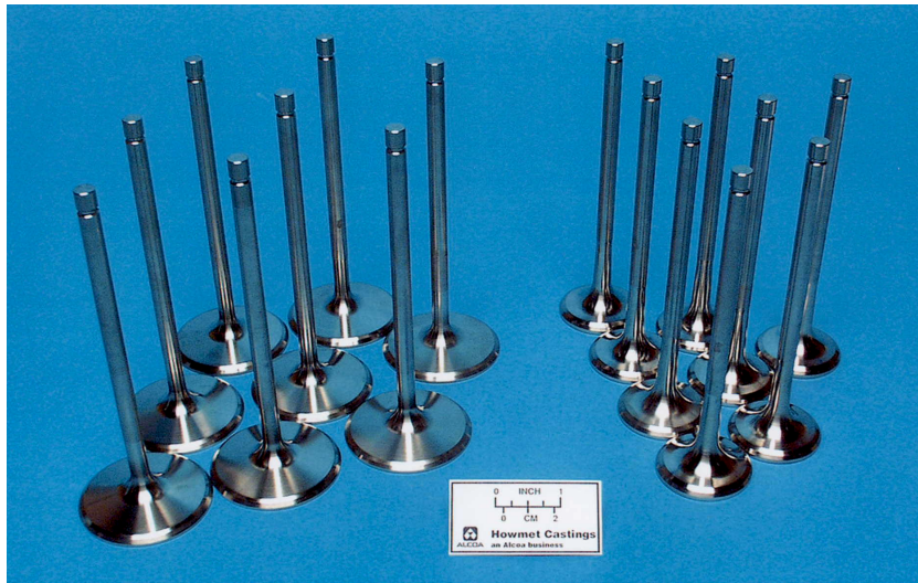
Figure 26: \gamma -TiAl automotive valves manufactured by Howmet Corporation. Courtesy of Howmet Castings.
