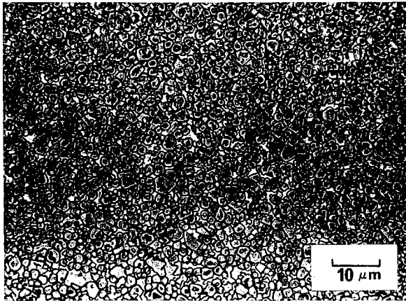
Figure 1. The microstructure of a typical steel cutting carbide tool.
