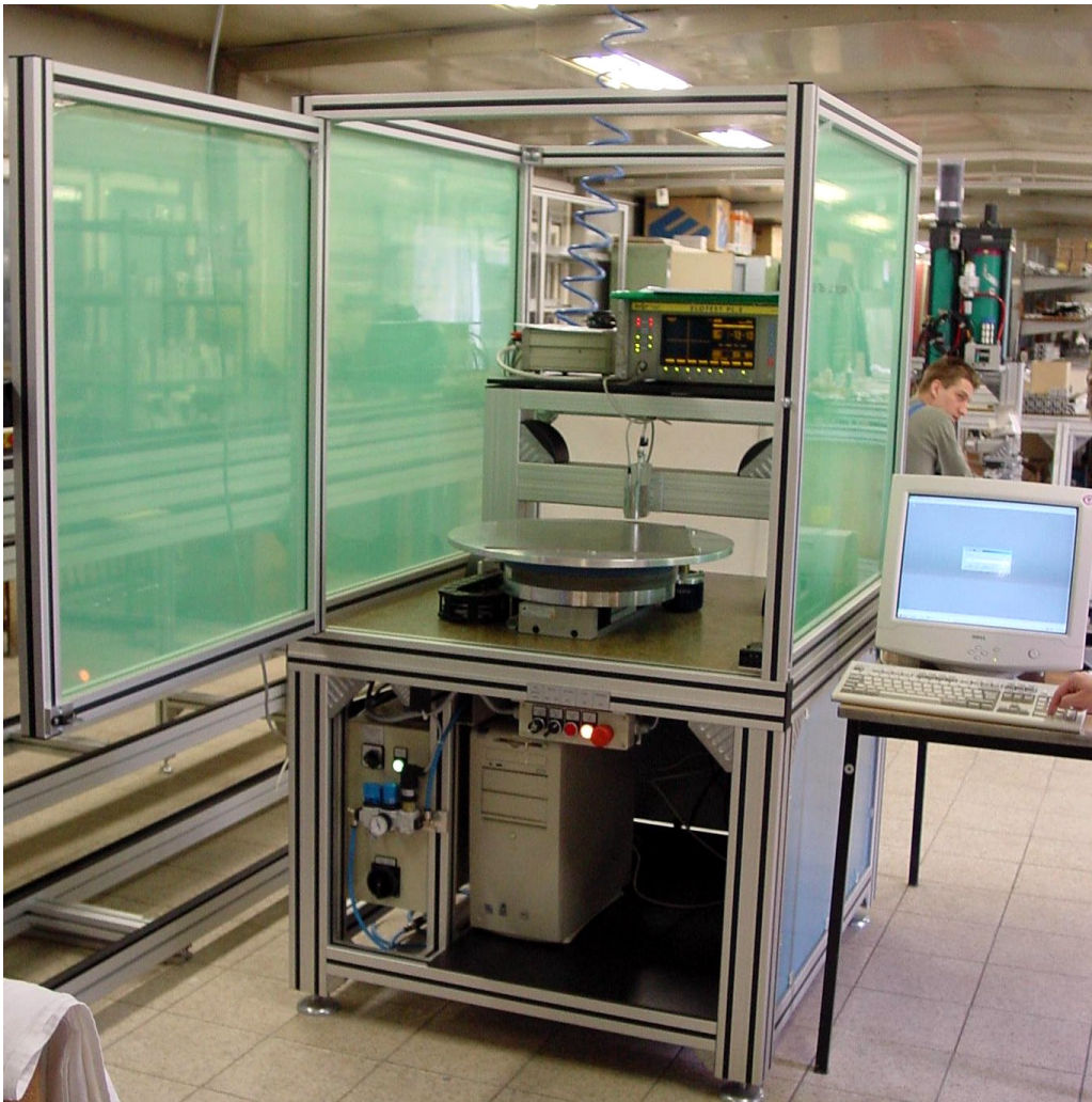
Figure 7: Eddy current scanning apparatus for niobium discs. This technology was developed by DESY and BAM (Bundesanstalt für Materialprüfung, Berlin). The above photo shows an equipment built for Jlab by the FER-PA GmbH (Forschung-Entwicklung-Rationalisierung), Magdeburg, Germany.
