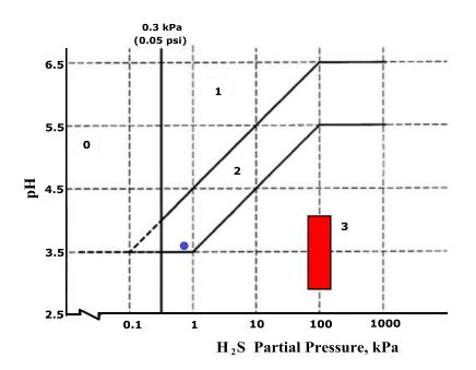
Figure 2. Severity of sour environments according to ISO 15156-2. The blue dot is the Petrobras' mean fluid condition in terms of pH and H<sub>2</sub>S partial pressure and the red rectangle is the standard test requirement [1].
