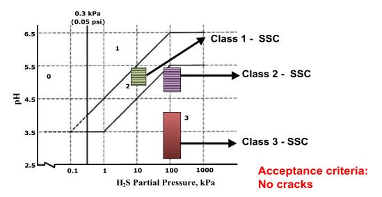
Figure 3. Petrobras class of corrosion severity.
