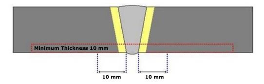
Figure 5. SSCC corrosion test specimen removal for girth weld joints. Weld toe shall be preserved from machining to evaluate HAZ transition.
