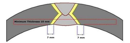
Figure 4. SSCC corrosion test specimen removal for DSAW linepipe weld seam. Weld toe shall be preserved from machining to evaluate HAZ transition.
