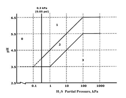
Figure 1. Severity of sour environment according to ISO 15156-2 [1].
