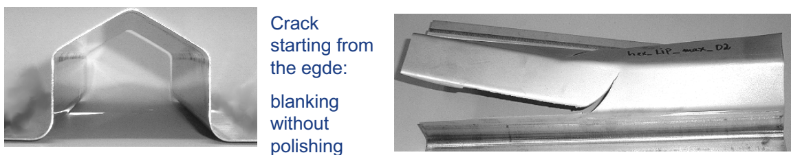
Figure 10. Stamping trials with cracks starting from the blanked edge of the sheets during the forming process.
