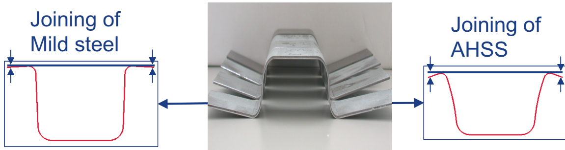
Figure 7. Springback comparison between mild steel and advanced high strength steel
