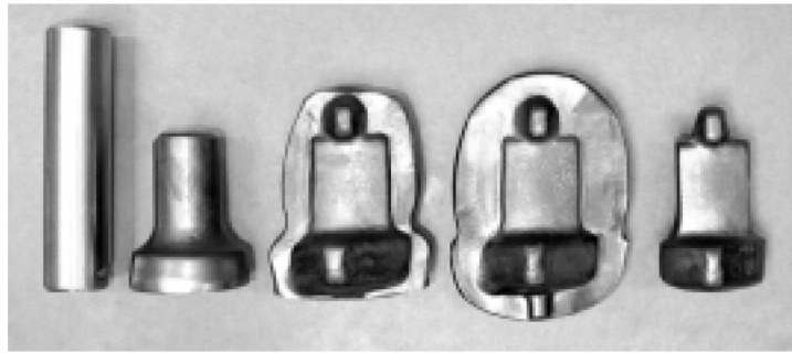
Figure 7: Process steps required to forge a near net shape blade from extruded bar
