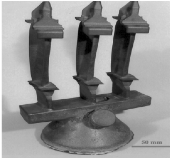
Figure 2: Cast trial of low pressure turbine blades in \gamma -TiAl at Birmingham University. Material used for this trials is the 45-2-2 alloy.
