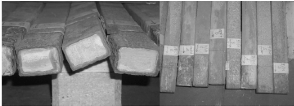
Figure 5: Extruded bars using stainless steel capsule technique in TNB alloy.
