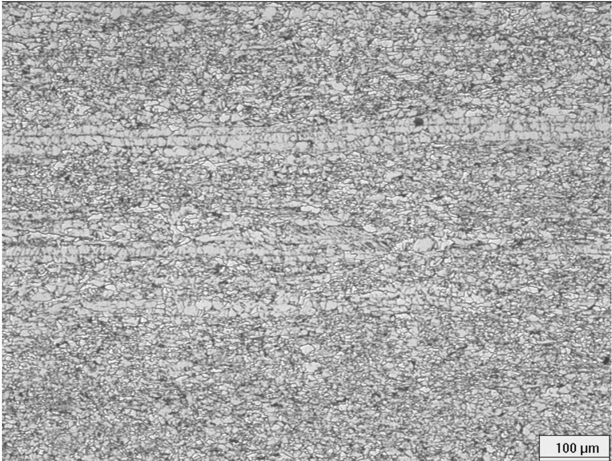
**Fig. 10 Optical micrograph of mixed grains**
