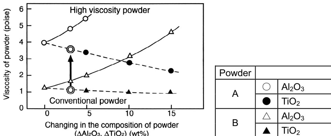
Figure 2. The effect of powder composition on the viscosity of molten powder.
