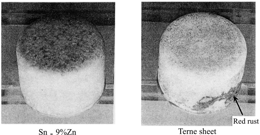
Figure 19. Anti-corrosion property of IF based Sn-Zn coated steel sheet.
