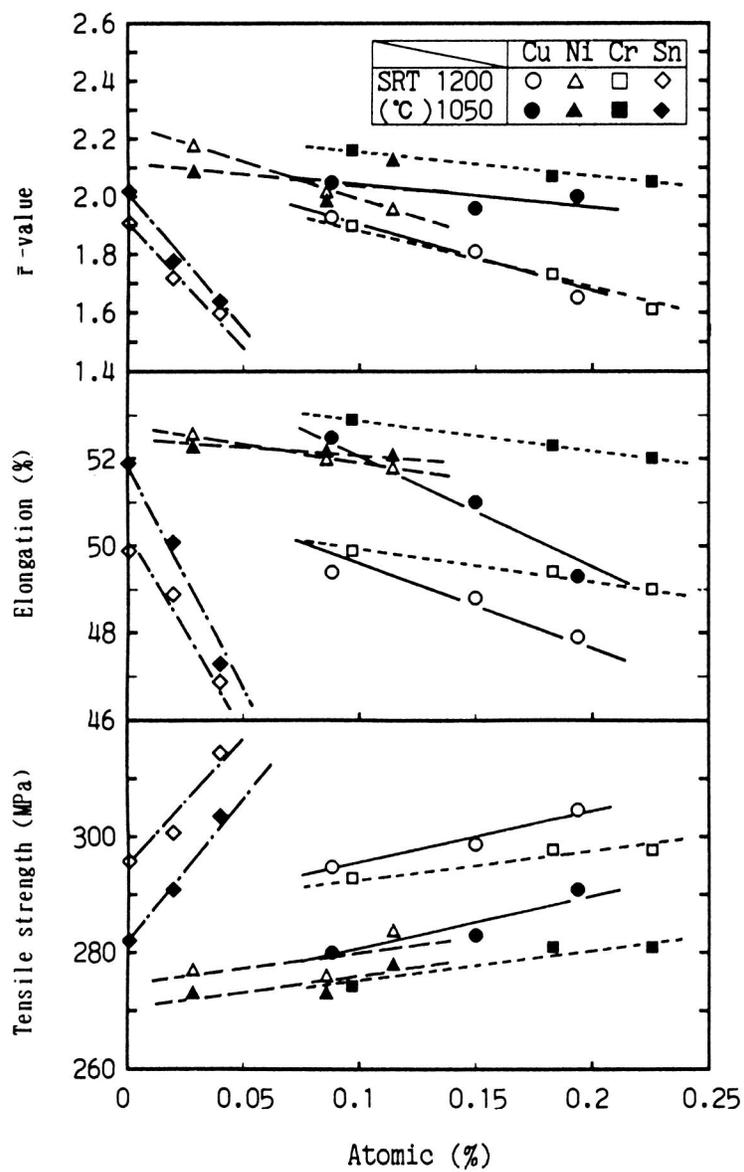
Figure 9. Relationships between atomic percent and mechanical properties of Cu, Ni, Cr and Sn-containing titanium-bearing extralow-carbon steel sheets [2].
