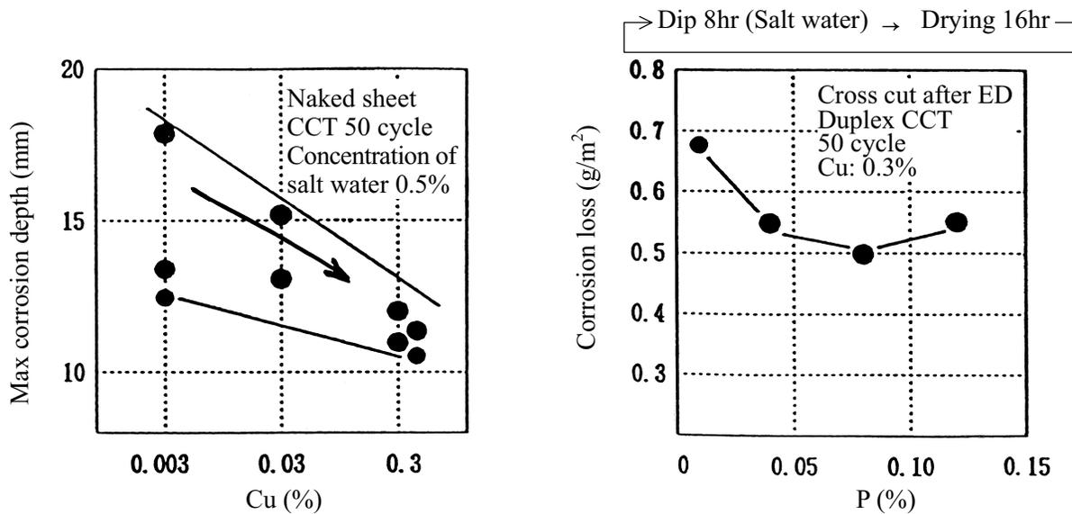
Figure 10. The effect of Cu and P on the corrosion resistant property.
