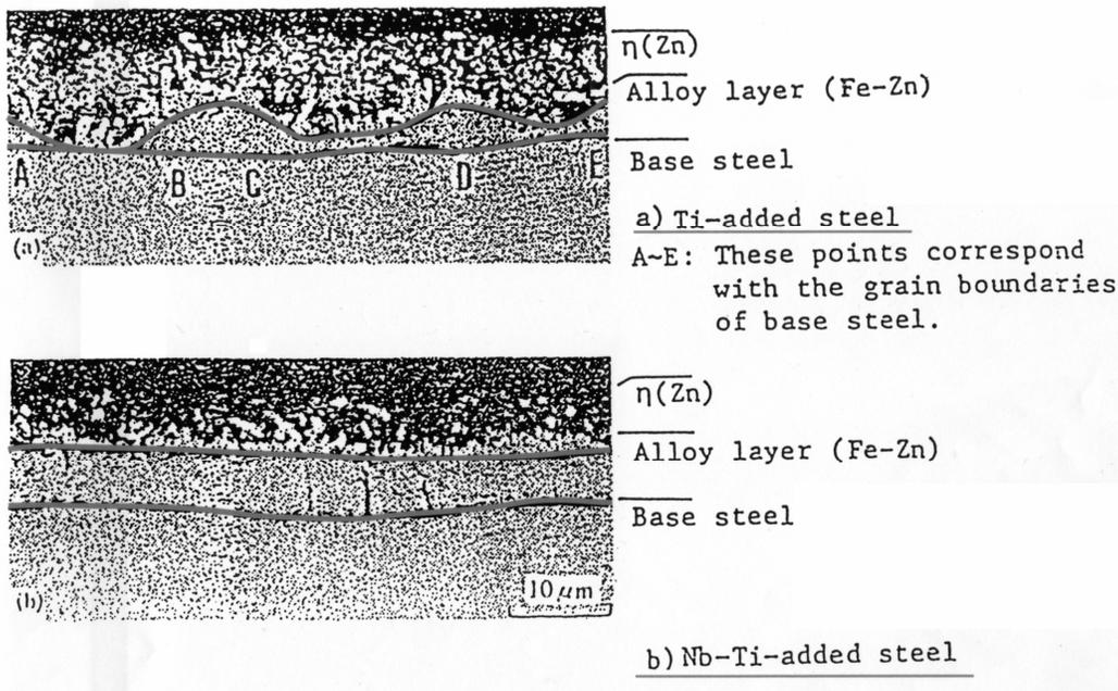
Figure 17. Alloy layer in the middle of growth [6].
