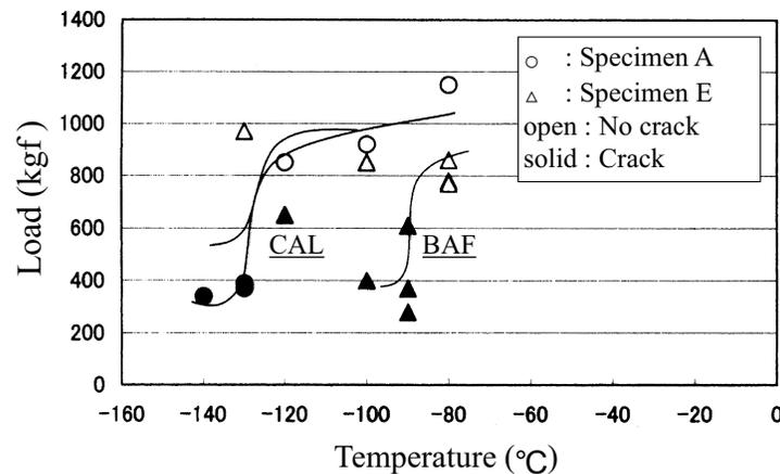
Figure 7. The relation between load and cracking, A and E are specimen No., CAL and BAF are continuous annealing and batch annealing respectively [1].
