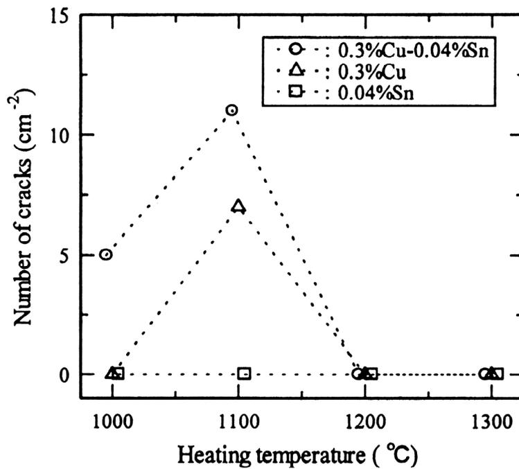
Figure 11. Effect of heating temperature on the surface cracking caused by Cu and Sn [3].
