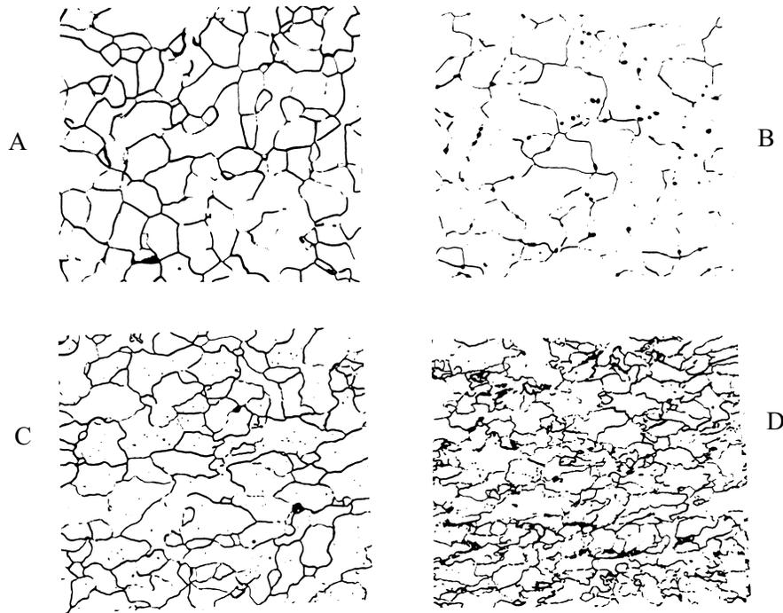
Figure 5. Microstructure of hot rolled steel [1].
