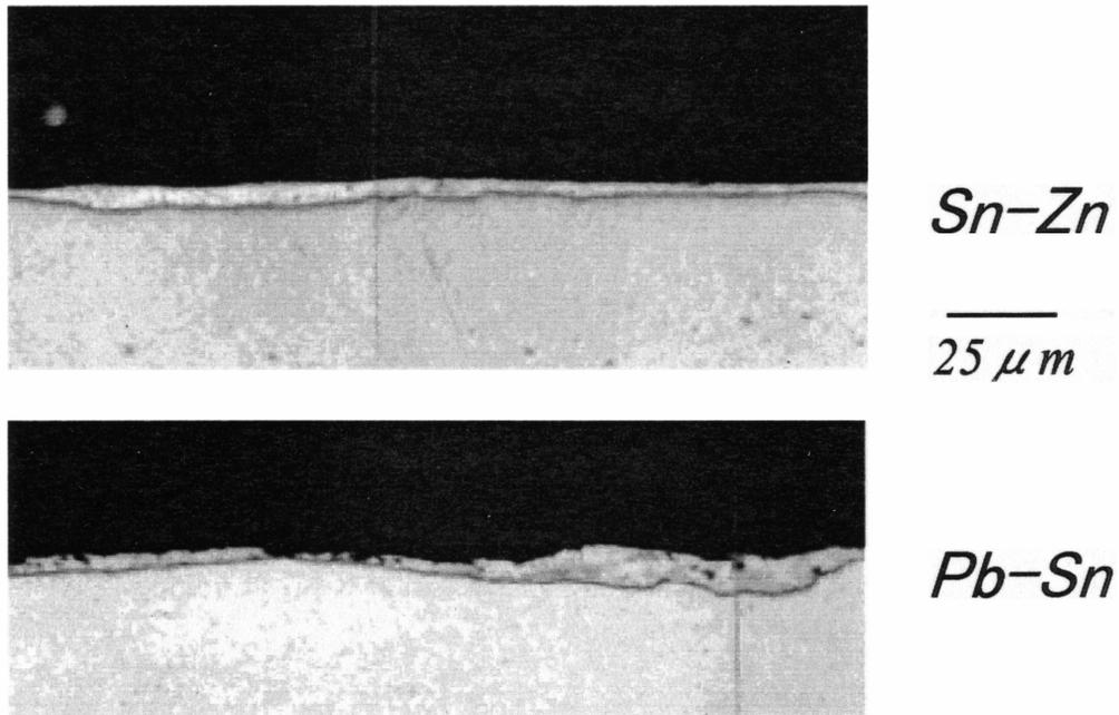
Figure 18. Damage of coated layer after draw-bead test.
