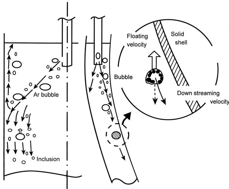
Figure 3. Origin of blow holes in slab casting.
