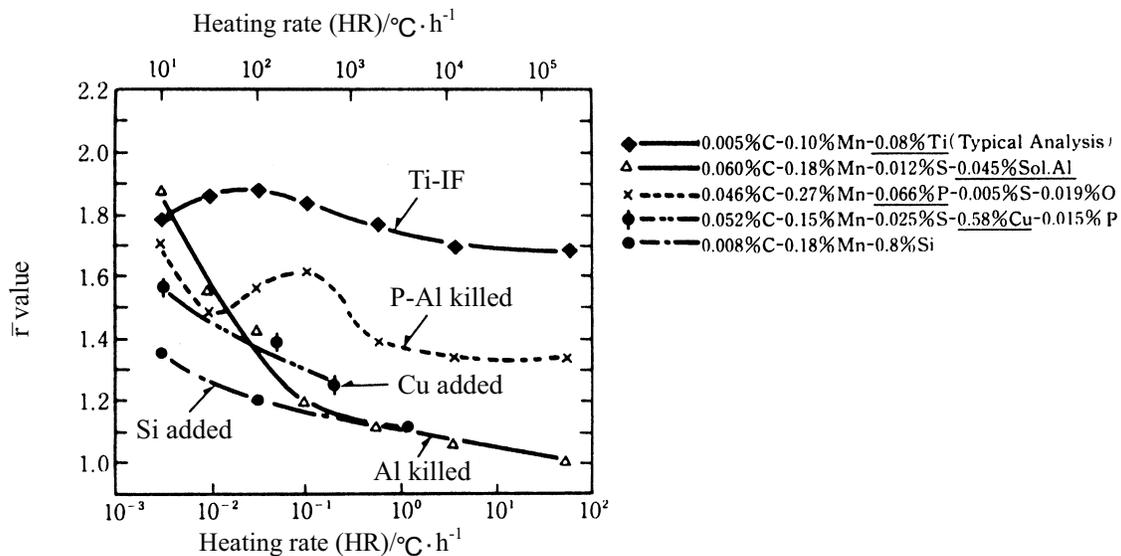
Figure 13. The effect of heating rate on  $\bar{r}$  value of steel sheet annealed at 700°C for 5 hrs [4].
