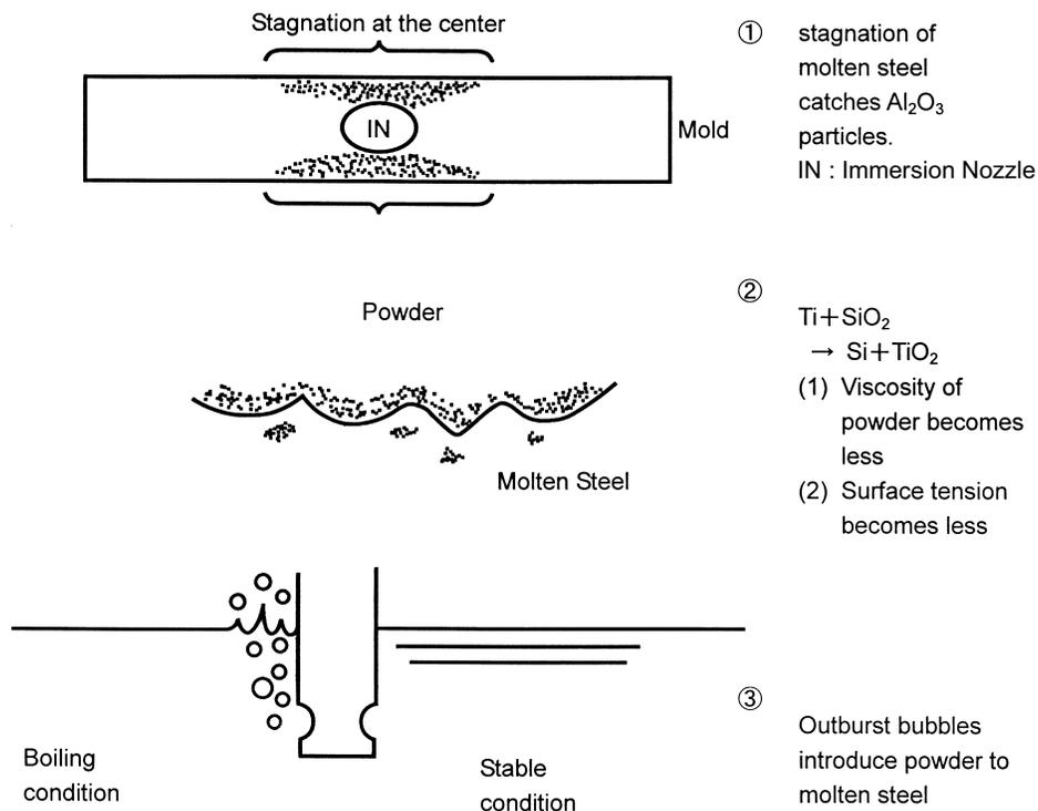
Figure 1. Origin of slivers in slab casting.
