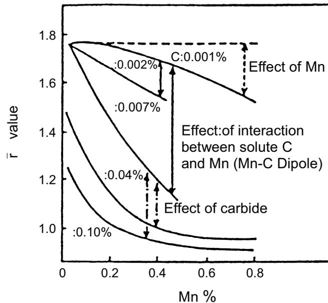
Figure 20. Schematic illustration of the effects of various metallurgical factors on the decrease in  $\bar{r}$ -value [8].
