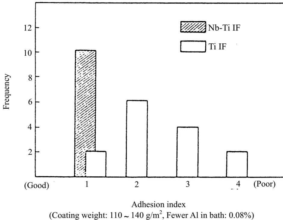
Figure 16. The effect of chemical composition on the adhesion of zinc coated layer [6].
