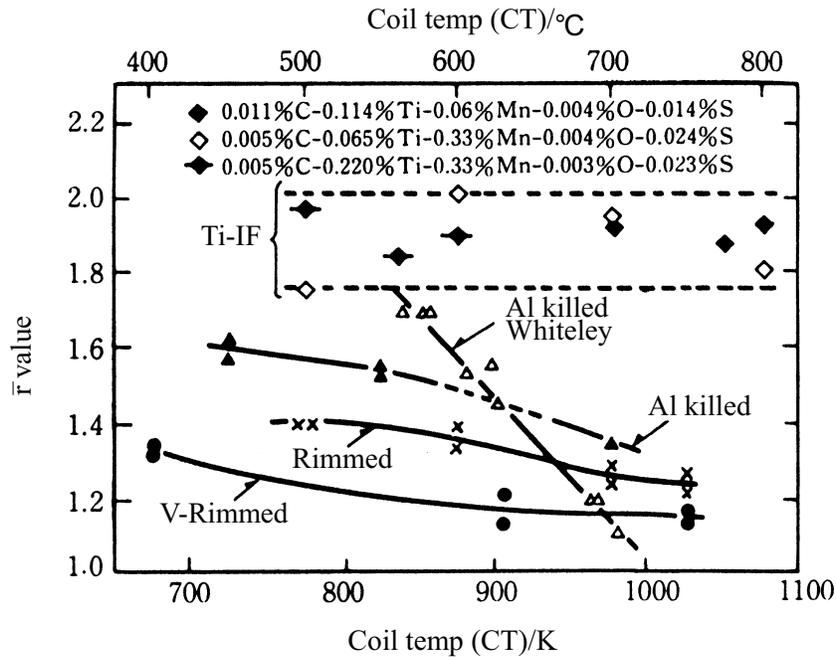
Figure 12. The effect of coiling temperature on  $\bar{r}$  value of steel sheet annealed at 700°C for 5 hrs [4].
