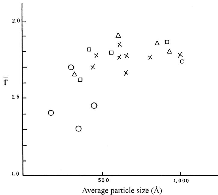
Figure 15. Relation between  $\bar{r}$  and average particle size of cold rolled-annealed sheets [5].
