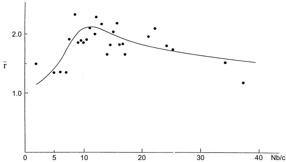
Figure 14. Relation between  $\bar{r}$  value and Nb/C of cold rolled-annealed sheets [5].
