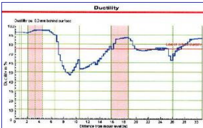
Figure 19. Ductility in the bending and straightening zone of CCM [19].
