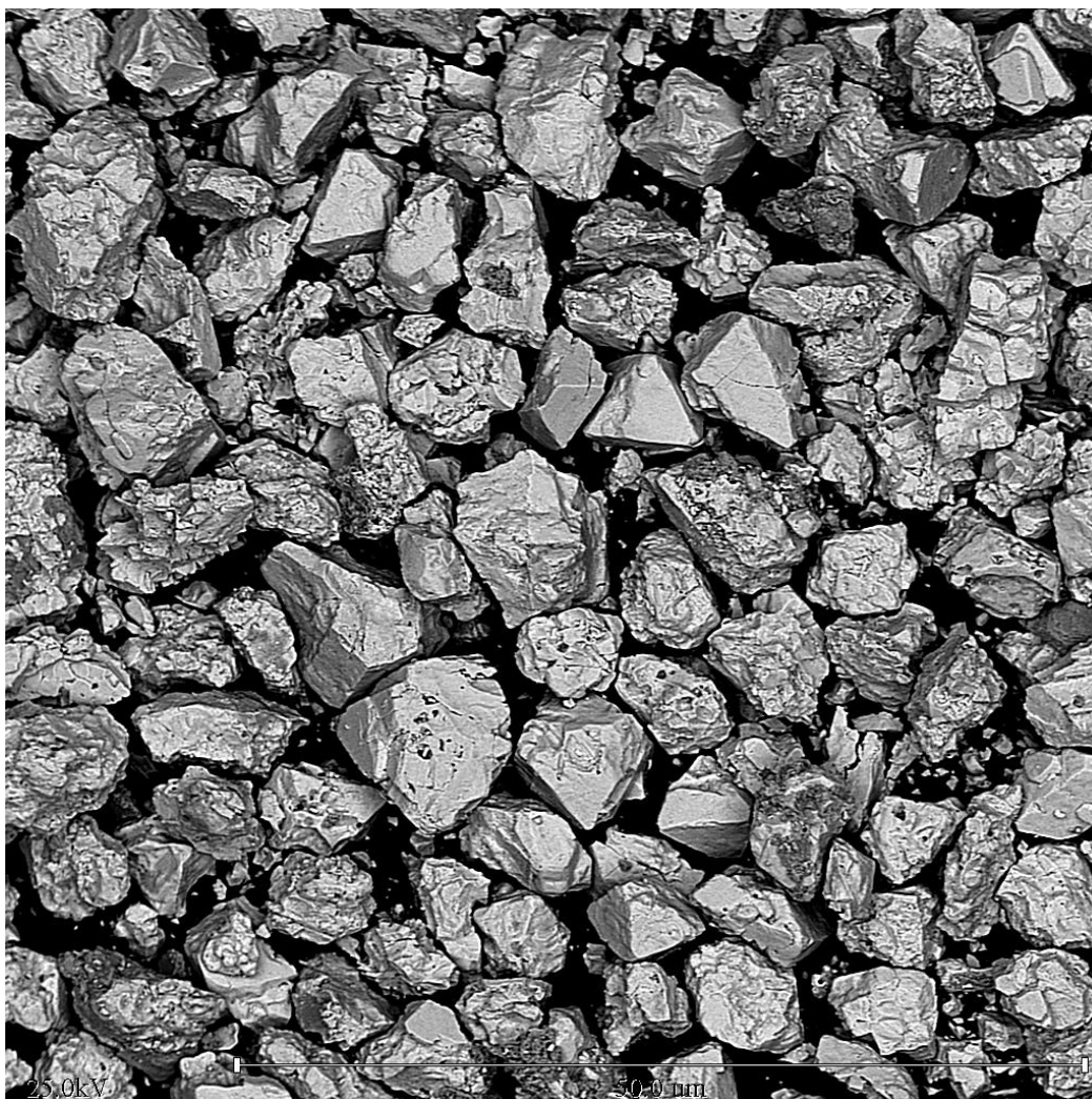
Figure 9: Floatation concentrate: bariopyrochlore retained on 200# Tyler sieve.
