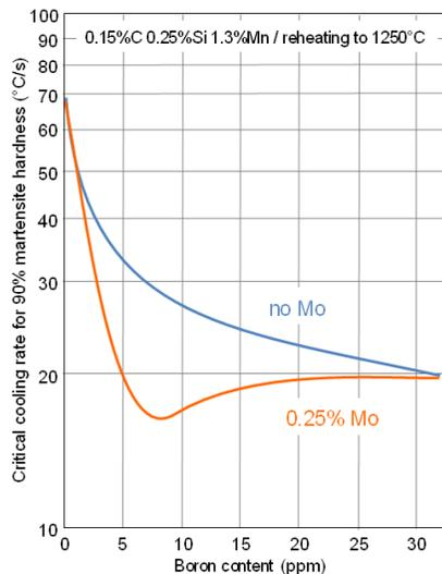
Figure 15. Influence of Mo on the effectiveness of B alloying with regard to the critical cooling rate to obtain 90% martensite hardness.
