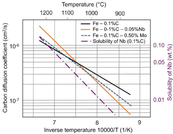
Figure 8. Solubility of Nb in 0.1%C steel and influence of solute Mo and Nb on the diffusivity of C.
