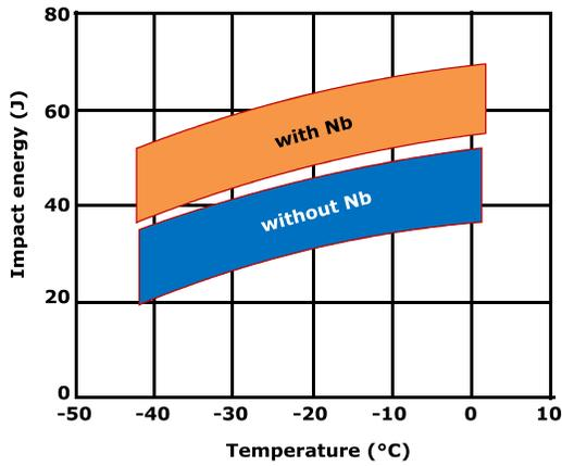
Figure 22. Toughness as a function of impact temperature for 450 HB abrasive resistant plate steels without and with Nb microalloying.
