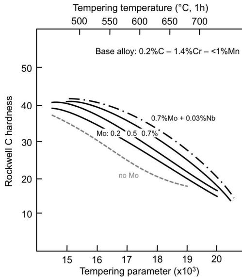
Figure 20. Effect of increasing Mo additions and Nb microalloying on the tempering resistance.
