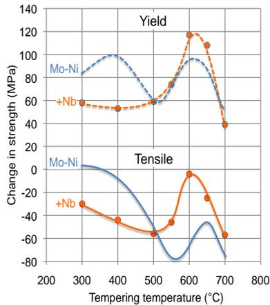
Figure 18. Influence of tempering temperature (30 min.) on the yield and tensile strength of 0.07%C-0.2%Mo-0.3%Ni steel and cross effects of Nb alloying.
