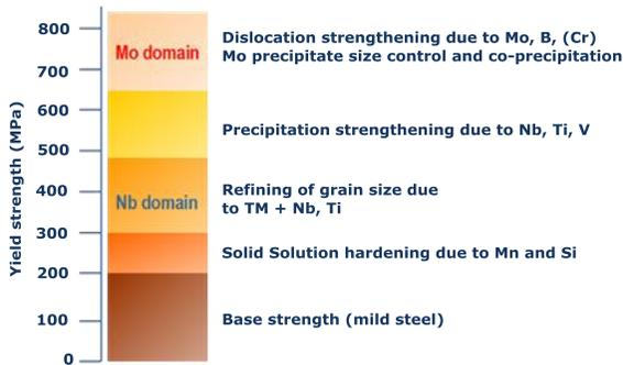
Figure 3. Strengthening effects in HSLA steel.
