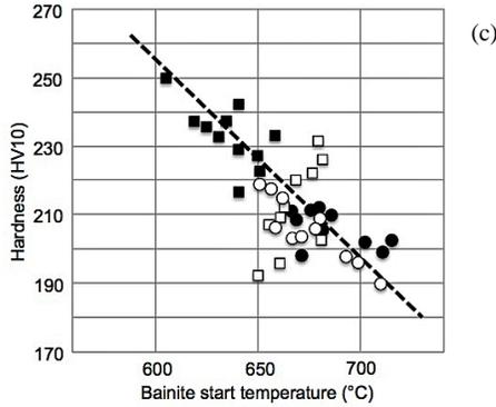
Figure 12. (a) Effect of Mo, Nb and B on bainite start temperature in 0.03%C steel at a cooling rate of 15 K/s, (b) bainite start and stop temperatures in 0.03%C steel; strain  $\epsilon=0.6$  at 850 °C; cooling rates: 1 – 15 K/s; Mo, Nb, B variable, other alloying elements constant, (c) hardness as a function of bainite start temperature (symbols correspond to (a)). All compositions in wt% except B ppm.
