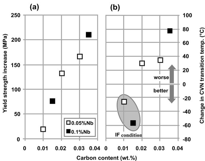
Figure 13. (a) Precipitation hardening effect after DQ cooling and subsequent tempering at 600 °C/1h in Mo-Nb ULCB steels, (b) corresponding change in the DBTT.
