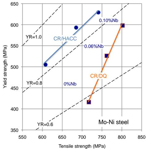
Figure 17. Influence of the cooling route on the strength of 0.07%C-0.2%Mo-0.3%Ni steel and effects of Nb alloying.
