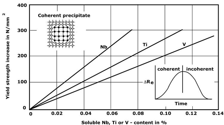
Figure 14. Strength increasing potential of microalloying elements by coherent precipitation.
