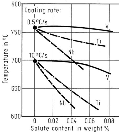
Figure 9. Effect of solute microalloying elements on the  $\gamma$ - $\alpha$  transformation temperature.
