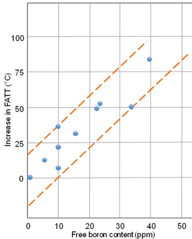
Figure 16. Influence of the free B content (not fixed as BN) on the fracture appearance transition temperature (FATT) in 0.10-0.12%C steels.
