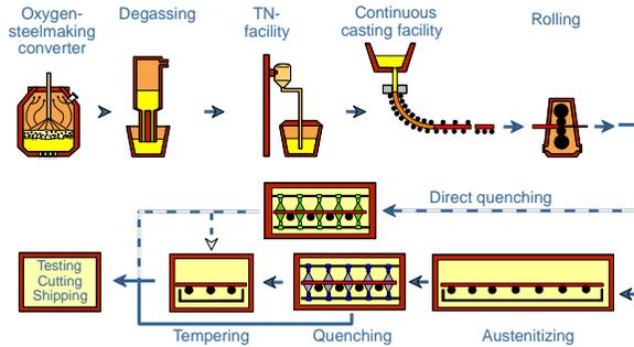
Figure 4. Processing routes for quenched and tempered steel.
