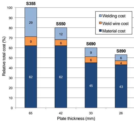
Figure 2. Material and welding cost of higher strength steels relative to S355.
