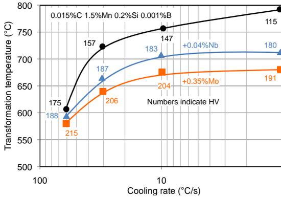
Figure 10. Effect of cooling rate on transformation temperature and hardness in ULCB steel with B, Nb-B and Mo-B alloying.
