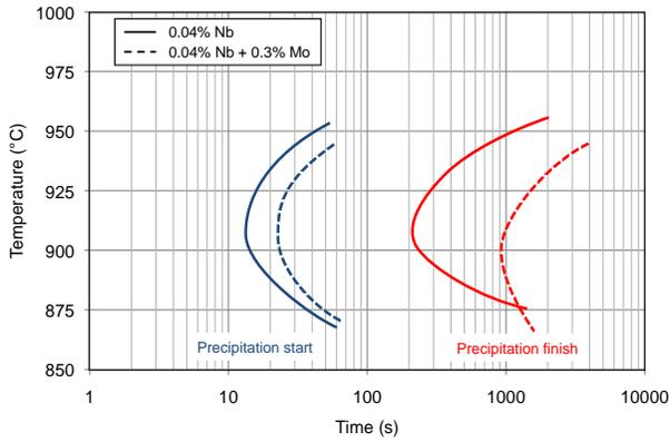
Figure 7. Influence of Mo addition on the strain induced precipitation behavior of Nb.
