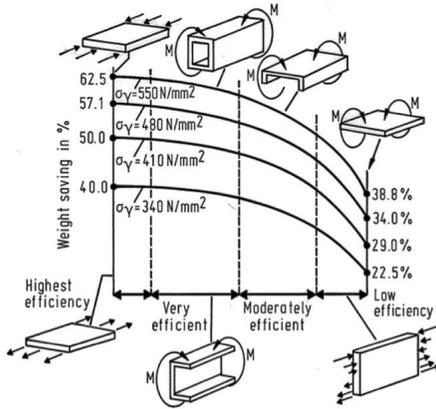
Figure 1. Weight saving potential by substituting 200 N/mm<sup>2</sup> steel with high strength steels for various loading conditions.
