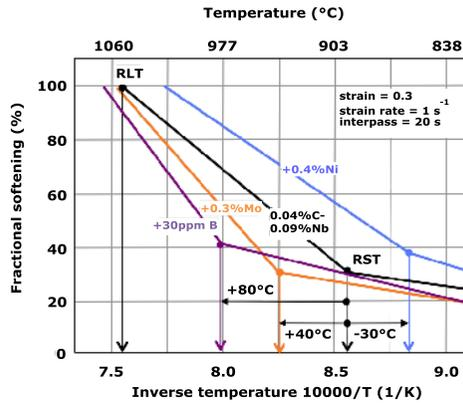
Figure 6. Effects of Mo, B and Ni addition to a low-C high-Nb base alloy on fractional softening behavior.
