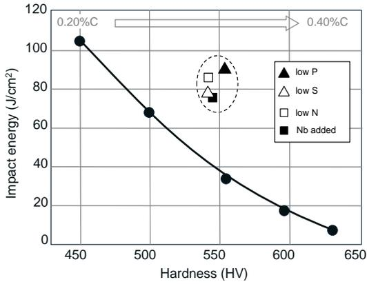
Figure 21. Dependence of impact toughness on hardness (C-content) of as-quenched martensite and metallurgical methods of increasing toughness.
