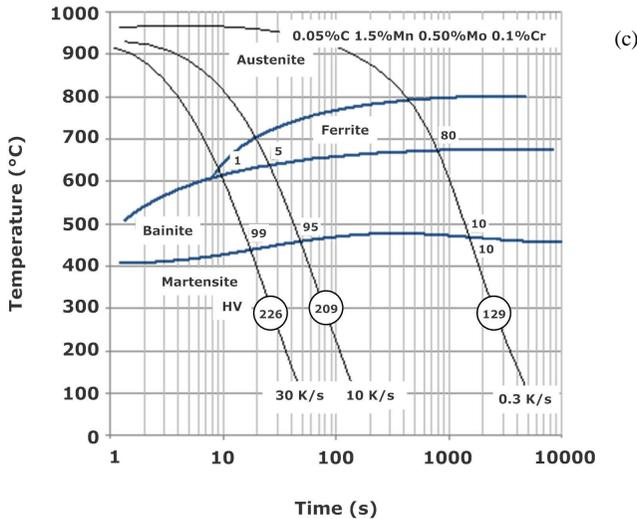
Figure 11. Effect of Mo alloying on the transformation behavior of a low-carbon base alloy (heating to  $A_{c3}+50$  °C – holding for 10 minutes without deformation – cooling at various rates): (a) 0.05% C, 1.5% Mn, 0.0% Mo, 0.1% Cr, (b) 0.05% C, 1.5% Mn, 0.25% Mo, 0.1% Cr, (c) 0.05% C, 1.5% Mn, 0.50% Mo, 0.1% Cr.
