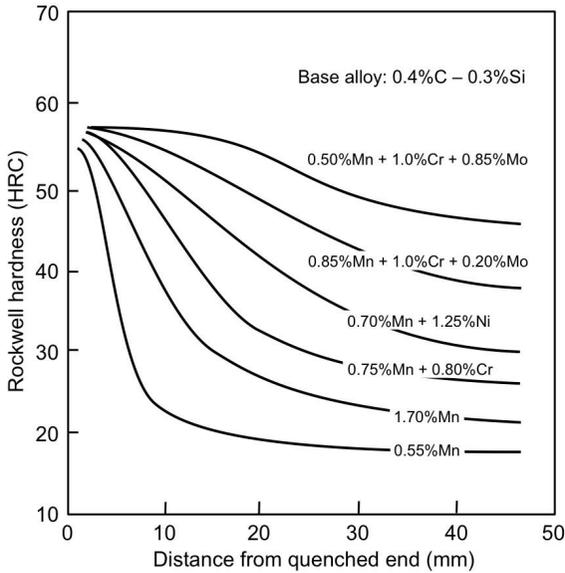
Figure 19. End quenching curves demonstrating the effect of various alloy combinations on through-hardenability.
