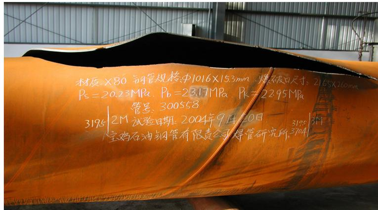
Figure 3.9 Burst Pipe
